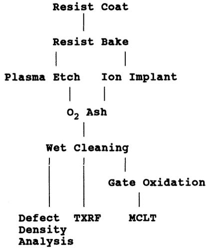
Figure 1. The test wafer process flow
