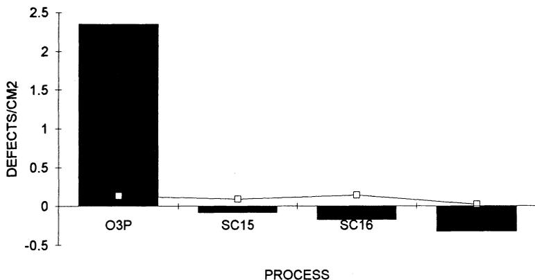
Figure 3. Defect density analysis of O3P versus heated SC1 processes for plasma etched samples
