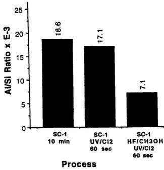
Fig. 4 SIMS results showing more effective removal of Al in the case UV/Cl<sub>2</sub> exposure was preceded by *in situ* etching of chemical oxide
