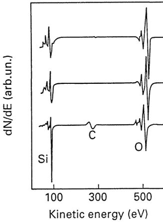
Fig. 3: Auger electron spectra before (top), during (middle) and after (bottom) etching of 100 nm SiO<sub>2</sub> on Si.
