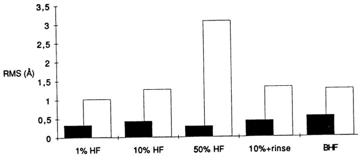
*Diagram 1.* The RMS-values of the surface roughnesses as measured in an AFM before and after each treatment.
