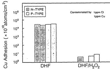
Figure 10 The effect of HF/H<sub>2</sub>O<sub>2</sub>/H<sub>2</sub>O (FPM) cleaning
