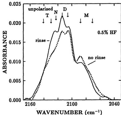
Fig. 6 : Comparison of the  $\text{SiH}_x$  absorption spectrum for a 5 min etching in 0.5% $\text{HF}/\text{H}_2\text{O}$  with and without rinsing.
