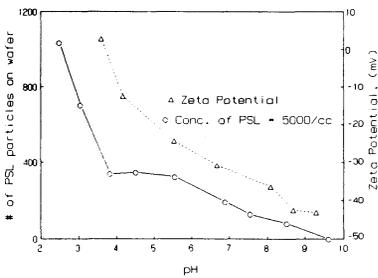
Fig. 5 Correlation between zeta potential values and PSL particle deposition on LPCVD nitride wafers cleaned by piranha.
