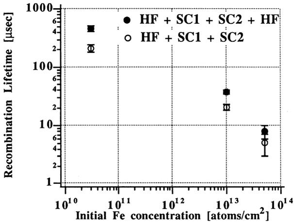
Figure 1. The plot of photoconductivity recombination lifetime of Si versus initial surface Fe coverage
