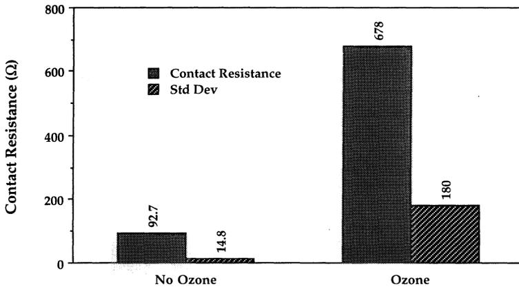
Figure 2. Effect of Rinse Water Type on Contact Resistance
