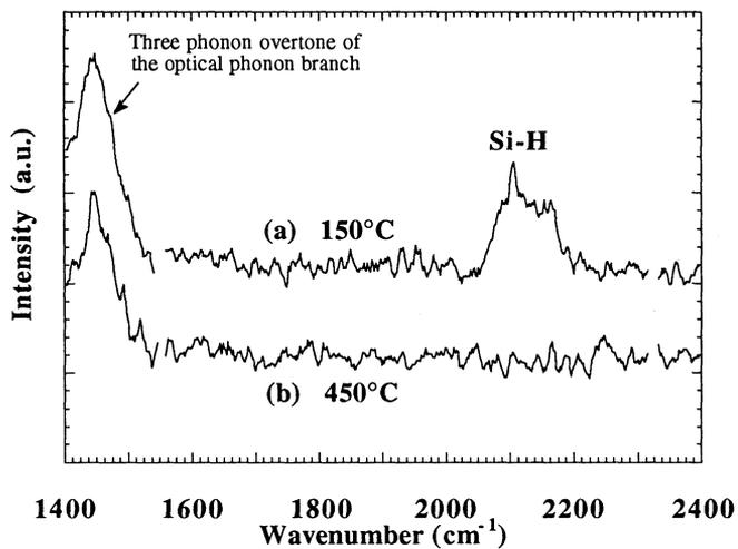
Fig. 5 Raman spectra collected from Si (100) following H-plasma exposure for 60 min at (a) 150°C and (b) 450°C. The feature at  $\sim 2100 \text{ cm}^{-1}$  is related to Si-H bonding in a Si crystal.
