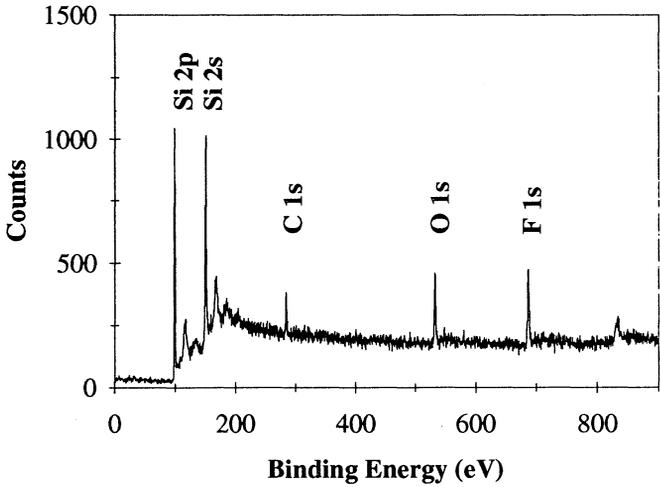
Figure 5 XPS spectrum of a sample that was UV/Ozone cleaned followed by an anhydrous HF etch.
