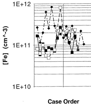
Fig. 7. [Fe] data from three spray processors. Levels settled to below 3E11 for all systems.
