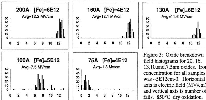
Figure 3: Oxide breakdown field histograms for 20, 16, 13,10,and,7.5nm oxides. Iron concentration for all samples was ~5E12cm-3. Horizontal axis is electric field (MV/cm) and vertical axis is number of fails. 850°C dry oxidation.
