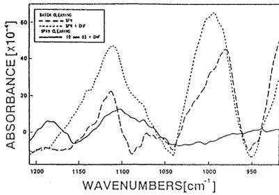
Figure 7 Native Oxide growth by spin cleaning and batch cleaning
