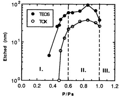
Figure 6. Etched thickness of thermal oxide and TEOS oxide as a function of the relative pressure ( $p/p_s$ ). The dotted lines indicate the different etch regimes: I. Gas phase, II. Enhanced adsorption and III. Condensation.
