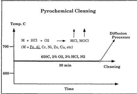
Figure 1. Schematic diagram of Pyrochemical cleaning process.
