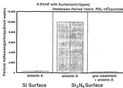
Figure 3 Prevention of particle deposition by surfactant for Si and Si<sub>3</sub>N<sub>4</sub> surfaces
