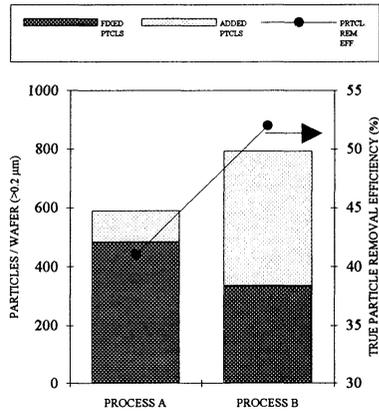
**Figure 3.** The particles of the processed wafers of fig. 2, classified as either fixed or added by PC software analysis of particle maps measured with the Censor ANS-100. The cleanliness of process A is superior, as shown by the smaller number of added particles. Process B is revealed to be better at removing particles.
