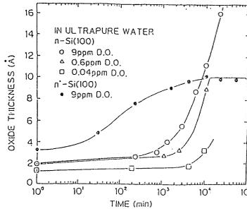
Figure 6 Native Oxide growth in ultra pure water under various dissolved oxygen concentration
