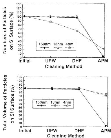
Figure 6. The removal efficiency of the Au ultra fine particles using various cleaning solutions.
