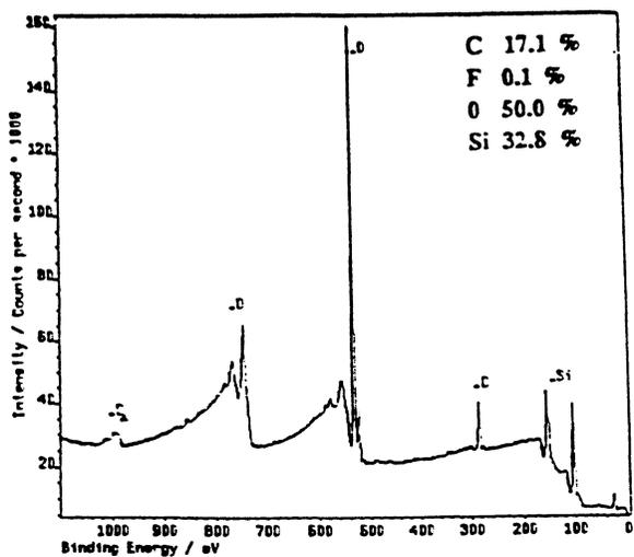
Figure 1(b). XPS results for the ECR oxygen cleaned sample from the RIE reactor using  $\text{CHF}_3$  chemistry.
