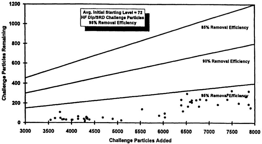
Figure 7. Particle removal efficiency of the MERCURY MP B Clean utilizing the Side Bowl Spray Post and ramped rinsing for 2 runs of 25, 150 mm wafers. The x axis indicates the number of “HF Last” challenge particles larger than  $0.15 \mu\text{m}$  added to a wafer. The y axis indicates the number of these added challenge particles remaining on the wafer after the clean.
