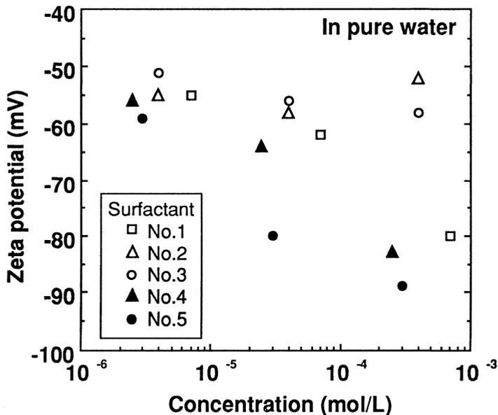
**Fig.1 Relationship between zeta potential of Si particle and concentration of various surfactants**
