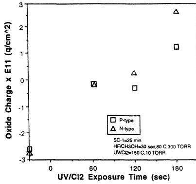
Fig. 7 Oxide charge vs. UV/Cl<sub>2</sub> exposure time with preceding oxide etching step.
