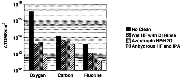
Fig. 7. SIMS data showing the effect of surface treatment on contamination levels at the tungsten silicide/Si interface.
