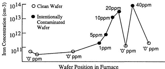
Figure 2: Effect of wafer position in furnace on resulting iron contamination. "Clean" wafers were interspersed among the intentionally contaminated wafers to monitor cross contamination within the oxidation process. Very little cross contamination of the clean wafers occurred.
