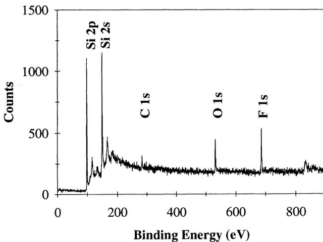
Figure 6 XPS spectrum of a sample that received the UV/Ozone clean followed by an anhydrous HF etch then a repeated 1 min UV/Ozone and HF etch clean.
