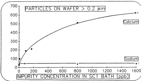
Figure 1: Calcium deposit in SC1, in particulate form
