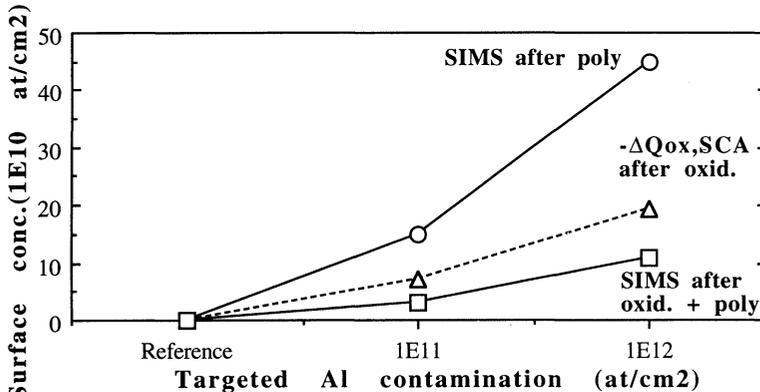
**Figure 1:** Surface concentration of: Al measured by SIMS on samples that have received poly deposition direct on silicon (o); Al measured by SIMS on samples that have received poly deposition on 15 nm oxide ( $\square$ ) and absolute fixed oxide charge shift measured by SCA on 15 nm oxides ( $\Delta$ ).
