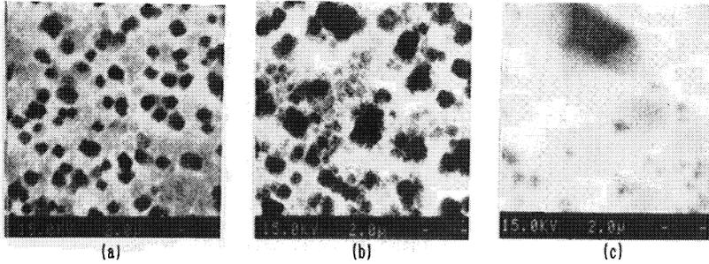
Fig.1 SEM photographs of the Si wafer surface after immersed in 630BHF for 24 hours at 25 °C. Wafer type is (a)P(100), (b)N(100), and (c)N(111).
