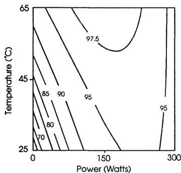
**Figure 3.** Contour plot of cleaning efficiency as a function of megasonic power and bath temperature with  $[\text{NH}_4\text{OH}]/[\text{H}_2\text{O}_2] = 1.0$
