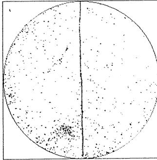
**Figure 7:** Typical LPD plot of a photoresist left half coated wafer that have received a high dose I/I, 45 min  $\text{O}_2$  plasma dry strip and 20 min SPM at 80  $^{\circ}\text{C}$  wet strip.
