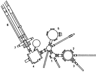
Fig. 1: Experimental set-up with load-lock (1), CVD chamber (2), HF/H<sub>2</sub>O etch chamber (3), RBS and AES analysis chamber (4), and XPS analysis chamber (5). The last stage of the RBS ion beam line (6) is indicated, including the spot-defining slit section (7).
