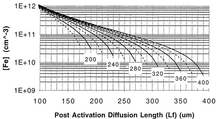
Fig. 8. Calculations of  $[Fe]$  versus post activation diffusion length value,  $L_f$  using Equ. [1]. Values of initial diffusion length are shown inset below their respective lines. Dashed lines are midpoint values, i.e.  $400 > 380 > 360$ . Length values are in micrometers.
