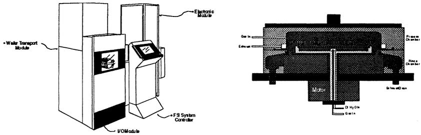
Figure 1: Vapor cleaning system and cross sectional diagram of process chamber.
