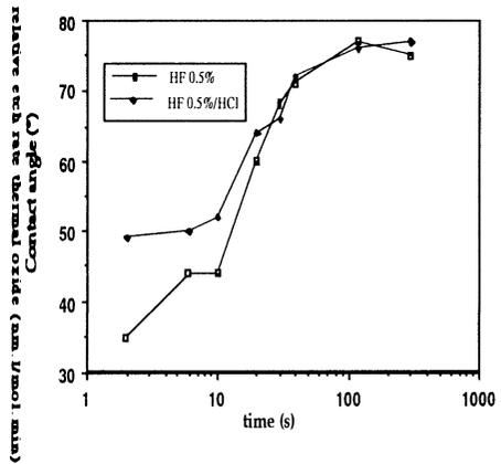
Figure 14 : Contact angle as a function of time for HF and HF/HCl mixtures.
