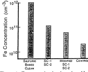
Figure 4: Fe contamination introduced by various cleaning chemistries. Note the control wafer had a starting iron concentration of  $2 \times 10^{10} \text{ cm}^{-3}$ .
