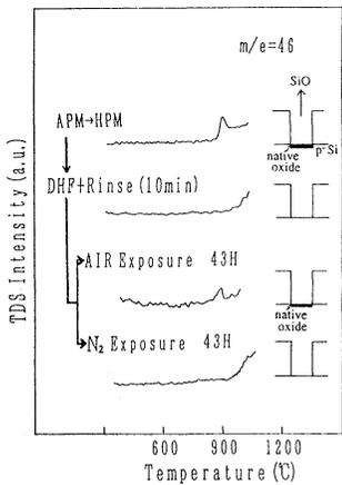
Figure 5 TDS spectra of SiO ( $m/e=46$ ) for contact-hole-bottom  $p$ -Si surfaces after cleaning, DHF dipping and preservation in one of two atmospheres.
