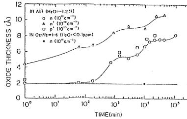
Figure 5 Thickness of native oxide grown in the air at room temperature as a function of time
