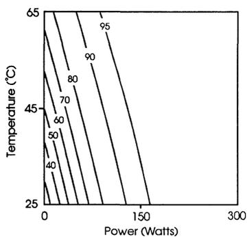
**Figure 1.** Contour plot of cleaning efficiency as a function of megasonic power and bath temperature with  $[\text{NH}_4\text{OH}]/[\text{H}_2\text{O}_2] = 0.01$
