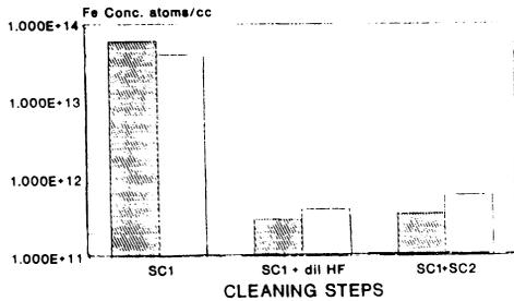
Fig. 4 The effect of various cleaning steps on the bulk contamination in p-type silicon following 1000C, 30 min. drive-in treatment in the nitrogen ambient.
