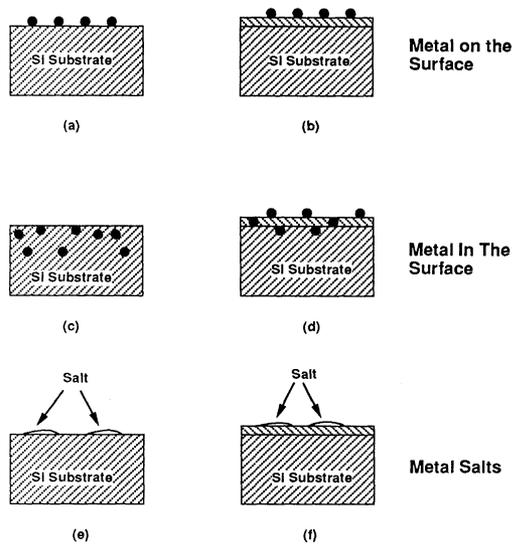
Figure 1. Schematic diagram of the possible locations of metals on a silicon surface. (a) represents metal atoms on a "clean" surface, which would be encountered if metal were deposited in ultrahigh vacuum; (b) represents the same case if a native oxide were present; (c) and (d) represent the case of a metal just below the surface; (e) and (f) represent the case of a metal salt deposited from solution.
