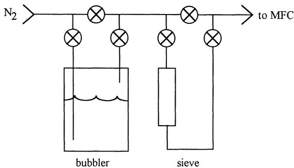
Figure 1. Schematic of bubbler/sieve manifold. Valves allow for the independent bypassing of the bubbler and/or the sieve.
