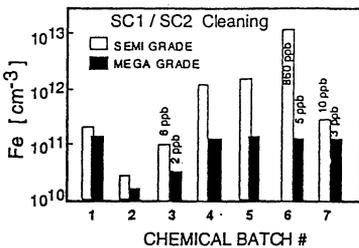
Figure 5: Fe contamination introduced during SC1/SC2 cleaning for different batches of SEMI and MEGA grade chemicals. Values of Fe in chemicals measured by ICPMS.
