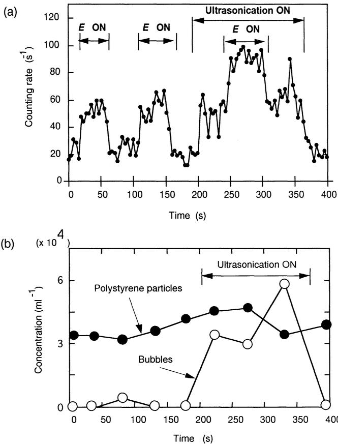
Fig. 6 Separate measurement of polystyrene particles and bubbles
