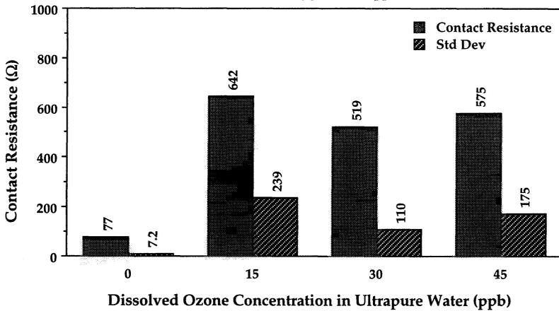
**Figure 6. Contact Resistance as a Function of Dissolved Ozone Level**
