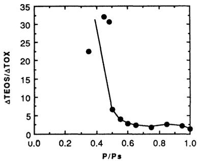
Figure 7. Etch selectivity as a function of the relative pressure. The selectivity is expressed as the ratio of etched thicknesses,  $\Delta \text{TEOS}/\Delta \text{TOX}$ .
