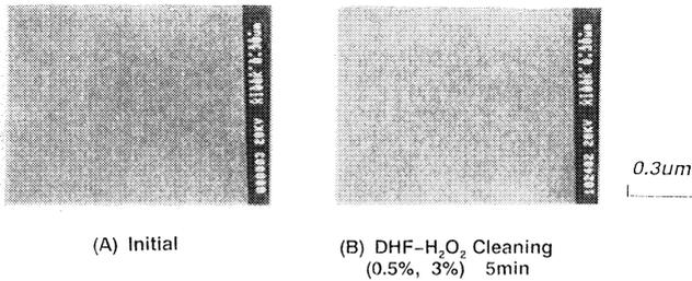
**Figure 8. SEM images of the sample wafer with Au ultra fine particles after DHF-H<sub>2</sub>O<sub>2</sub> cleaning. No obvious differences was observed.**
