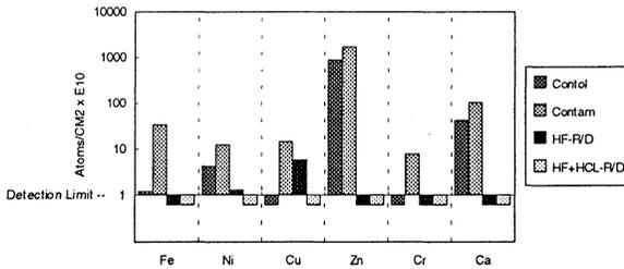
Figure 9: The effect of various vapor cleans on surface metallic contamination.
