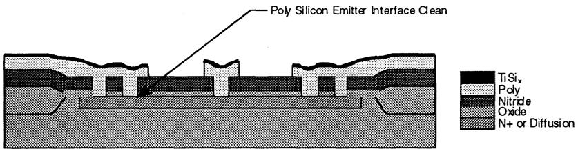
Figure 2: Cross section of diode test structure used for study of pre polysilicon deposition cleans.
