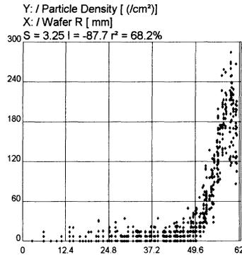
**Figure 9.** The radial distribution of the stacking faults on the wafer in fig. 8.
