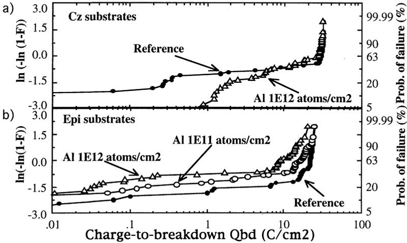
**Figure 6:** Charge-to-breakdown ( $Q_{BD}$ ) plots obtained with a current density of  $0.1\text{A}/\text{cm}^2$  for  $15\text{ nm}$  gate oxide capacitors that have received Al contamination. The results of ( $\bullet$ ) reference, ( $\circ$ )  $10^{11}$  atoms/ $\text{cm}^2$  and ( $\Delta$ )  $10^{12}$  atoms/ $\text{cm}^2$  nominal contaminated samples are shown for (a) Cz and (b) Epi substrates.
