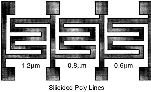
Figure 7: Constant length resistor bridge for measuring sheet resistivity.
