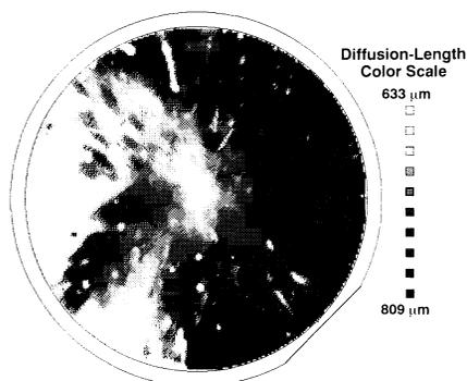
**Figure 1.** An ELYMAT diffusion-length map of a silicon wafer cleaned in a chemical spray tool and annealed at 650°C for 30 minutes. The effect of the spin-dry is clearly visible.
