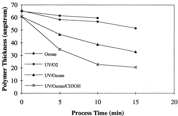
Figure 2 Removal of the RIE polymer as shown by the decreasing thickness of the polymer film as measured by ellipsometry using a constant index of refraction of 1.465.
