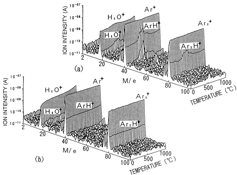
Fig. 4 APIMS-TDS spectra of (a) HF-cleaned silicon surface and (b) background.  $M/e=2-100$ , Temperature=RT-1000°C.
