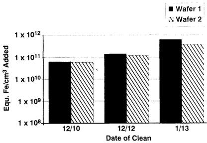
**Figure 3.** Monitor reuse investigated with two monitor wafers run through identical clean/anneal/measurement cycles.
