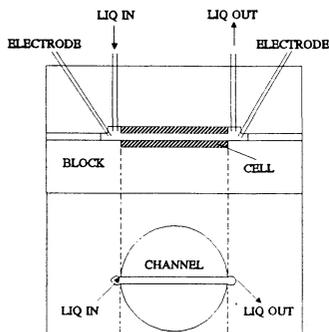
Fig. 1 A schematic sketch of the streaming potential cell for 5" wafers.
