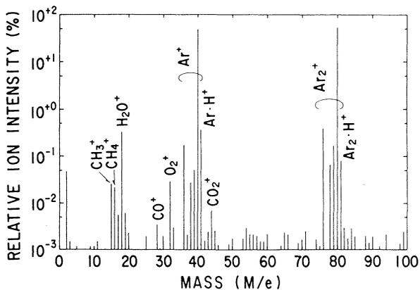
Fig. 3 APIMS spectra after gas purification. This condition corresponds to just before TDS analysis.
