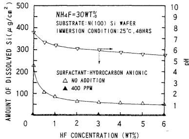
Fig.5 Dependence of pH and the amount of dissolved Si after immersed in BHF on the HF concentration in BHF.
