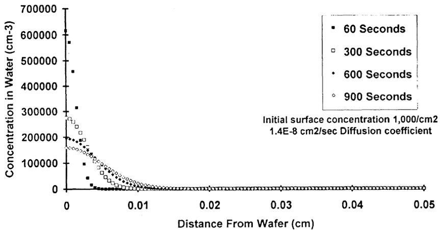
Figure 5. The calculated concentration of 0.3  $\mu\text{m}$  particles that have diffused away from the surface of the wafer in stagnant rinse water for diffusion times of 60, 300, 600 and 900 seconds.
