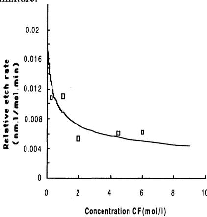
Figure 9 : Modelling of the relative etch rate of poly-Si as a function of fluoride concentration  $C_F$  in the case of a HF solution.
