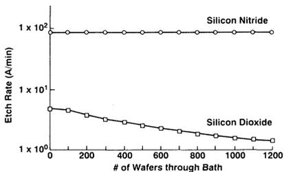
**Figure 2. Silicon nitride and silicon etch rates as a function of number of wafers through the phosphoric acid bath.**
