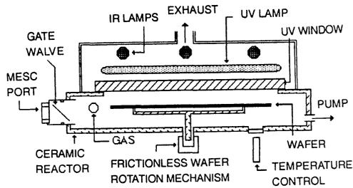
Fig.1 Schematic cross section of the reactor used in this study (5).
