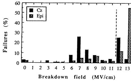
**Figure 3:** Breakdown field ( $E_{BD}$ ) histograms for 15 nm gate oxide capacitors fabricated on Cz (full bars) and Epi substrates (dashed bars). The dashed line indicates the yield criteria of 12 MV/cm.
