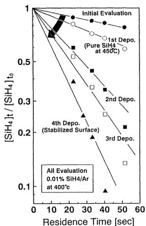
Figure 1 The thermal decomposition characteristics of  $\text{SiH}_4$  with the surface condition transition.
