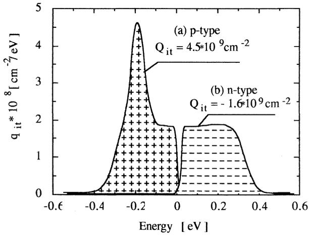
Fig. 4. Energy distribution of combined surface state charge resulting from SiO<sub>2</sub>/Si interface and iron contamination for (a) p-type and (b) n-type silicon.
