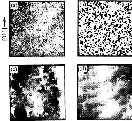
Fig. 6. AFM image ( $4 \times 4 \mu\text{m}^2$ ) of  $\text{H}_2$  annealed Si(100) surface after  $\text{H}_2$  annealing with various annealing temperatures, (a)  $800^\circ\text{C}$ , (b)  $900^\circ\text{C}$ , (c)  $1000^\circ\text{C}$ , (d)  $1100^\circ\text{C}$ .
