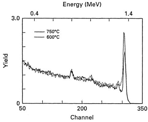
Fig. 5: Channeling-RBS spectra of LPCVD Si, deposited at 600 °C and 750 °C on Si(001).
