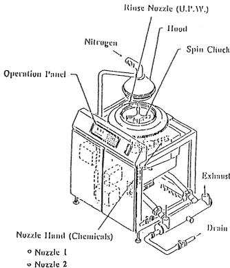
Figure 3 Nitrogen Gas Sealed - Advanced Spinner System
