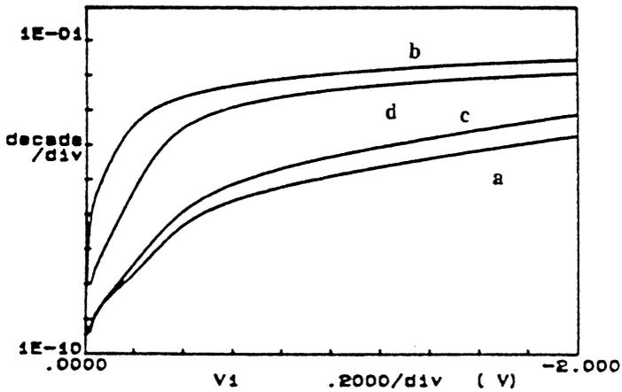
Figure 3. I-V curves for (a) an etched sample, (b) a control sample, (c) an etched and oxygen cleaned sample, (d) an etched, oxygen cleaned and HF etched sample for the MERIE  $\text{CHF}_3/\text{CF}_4/\text{Ar}$  case.
