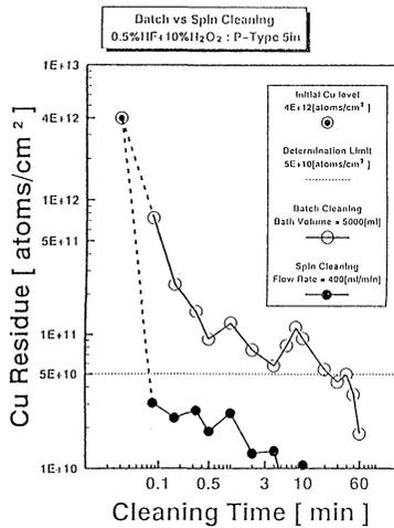
Figure 9 The cleaning time dependence on Cu removal efficiency with the spinning method and the batch method
