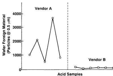
**Figure 3. Comparison of phosphoric-acid vendors and corresponding wafer foreign material levels.**
