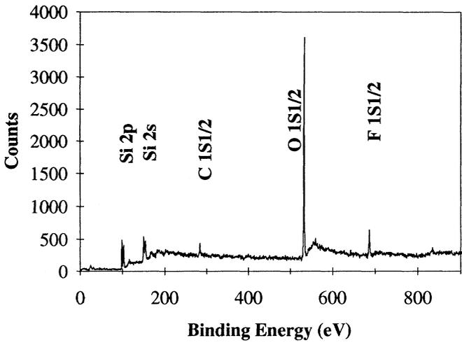
Figure 4 XPS spectrum of a sample after the UV/Ozone with the addition of methanol (CH<sub>3</sub>OH). (Note the change in the vertical scale)
