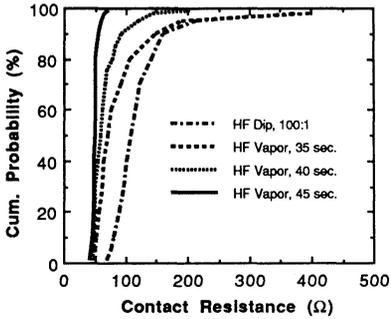
Figure 9. The contact resistance distribution between mono-Si and poly-Si for  $1.3 \mu\text{m}^2$  contacts. HF dip indicates a conventional process including a liquid oxide removal step. The etch times are varied from 35 to 45 seconds.
