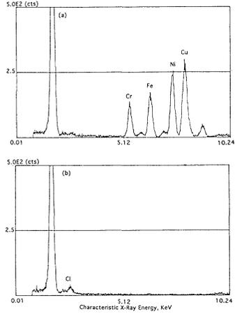
Figure 2. TXRF spectra of Fe, Ni, Cr and Cu intentionally introduced on a wafer (a) before and (b) after Pyrochemical Cleaning.
