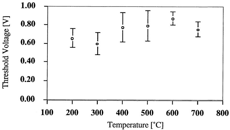
Figure 4. Plot of threshold voltage,  $V_t$ , vs. substrate temperature during H-plasma cleaning .
