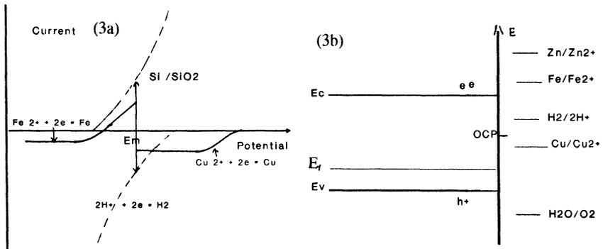
Fig.3a. Schematic mixed potential model for the metallic contamination of silicon.
