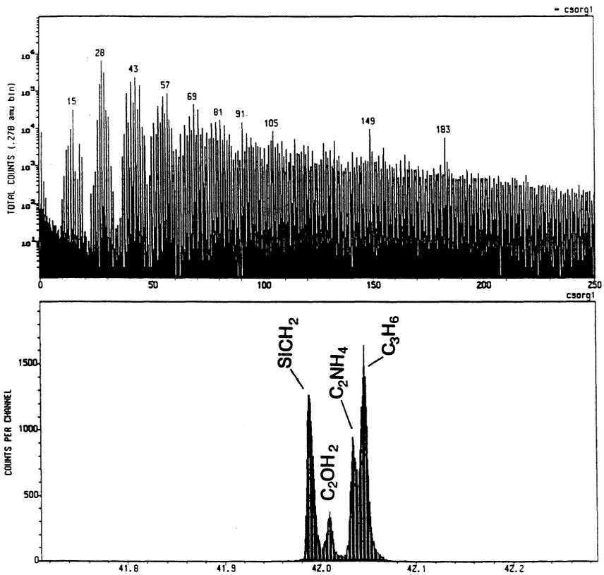
**Figure 4.** Positive secondary ion mass spectrum obtained from the surface of a silicon wafer. The Cs primary ion dose was approx.  $10^{11}$  cm<sup>-2</sup>. Figure 4a shows a logarithmic display of the mass spectrum in the mass range from 0 to 250 $\mu$ . Figure 4b is an expanded section of the same mass spectrum showing the signals around mass 42 $\mu$  with their respective identification.
