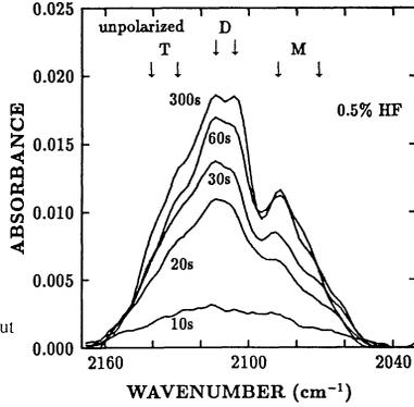
Fig. 2 : MIR spectra of the  $\text{SiH}_x$  stretching modes as a function of the etching time in a 0.5%  $\text{HF}/\text{H}_2\text{O}$  solution. Mono- (M), di- (D) and tri- (T) hydride peaks can be distinguished.
