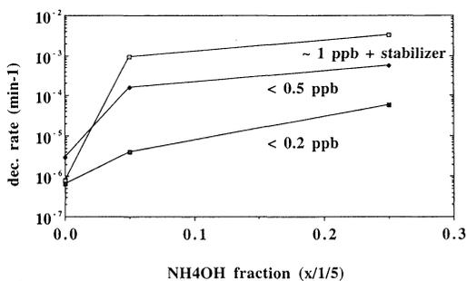
Figure 3: Decomposition rate of three different grades of H<sub>2</sub>O<sub>2</sub> as a function of the NH<sub>4</sub>OH/H<sub>2</sub>O<sub>2</sub>/H<sub>2</sub>O ratio at 70 °C (metal concentrations in total SC1).
