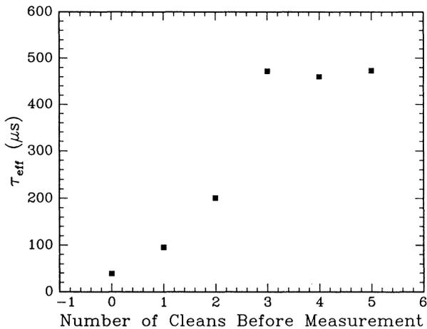
Fig. 2: Variation of measured lifetime with number of cleans for a contaminated phosphorous-doped float zone Si(111) to a resistivity of 2.66  $\Omega\text{-cm}$ . The wafer is 5 cm in diameter and 520  $\mu\text{m}$  thick.
