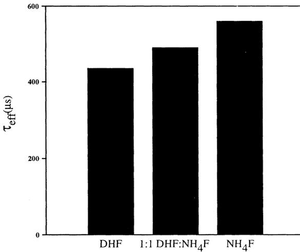
Fig. 7: Variation of lifetime with etch solution showing the correlation between surface roughness and measured lifetime.
