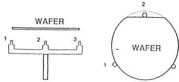
Figure 4 Teflon Chuck for Wafer
