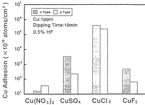
Figure 7 Cu contamination by various salts
