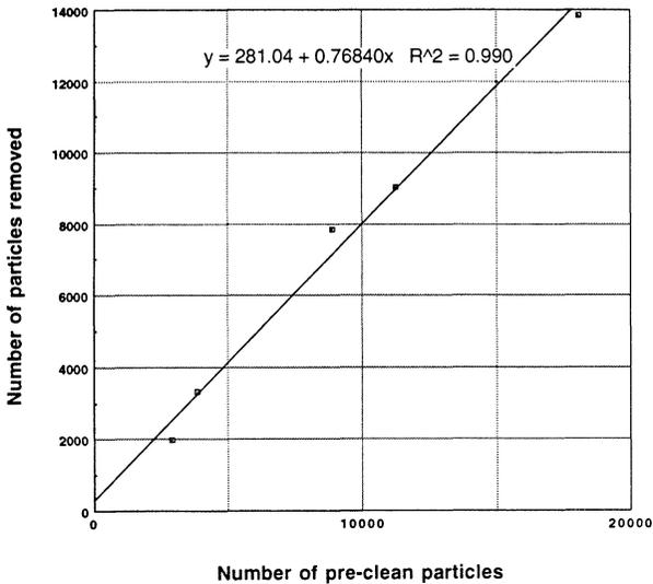
Fig. 1. Number of particle removed as a function of number of pre-clean starting particle counts for one of the 30 Catalyst test runs. The set points were megasonic cleaning power of 300 W and time of 10 min., 7 quick dumps, rinse power of 100 W and time of 15 min. The slope of the line was used as the Figure of Merit.
