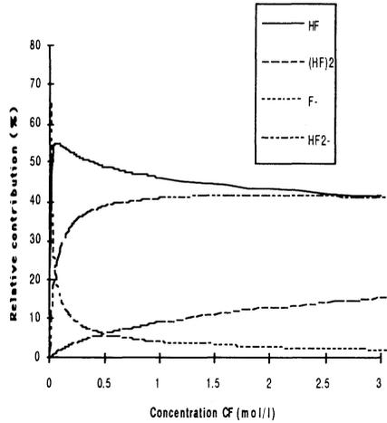
Figure 10 : Relative contributions to the etch rate of poly-Si as a function of fluoride concentration  $C_F$  in the case of a HF solution.
