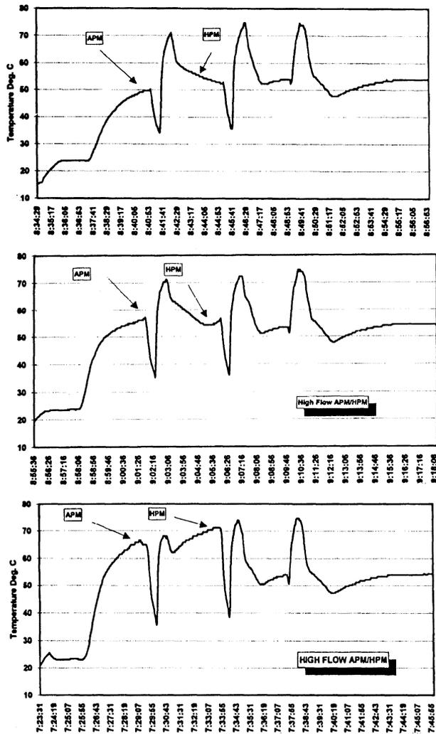
Figures 1a - 1c. On-wafer temperatures traces for two, 4 minute dispenses of DI water with each followed by brief cold and hot rinses. Dispense flow rates were set to simulate the chemical dispenses: a) 1650 cc/min with in-line heater inactive. b) 2400 cc/min with in-line heater inactive. c) 2400 cc/min with in-line heater active at 95°C set point.
