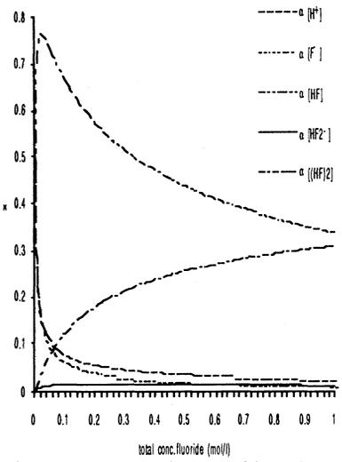
Figure 2 : Calculated composition of the HF mixture as a function of total fluoride concentration, when taking the dimerisation reaction into account.
