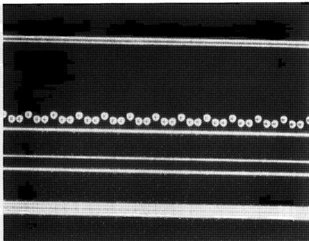
**Figure 5.** Optical dark-field microscopy photograph showing phosphoric acid haze.
