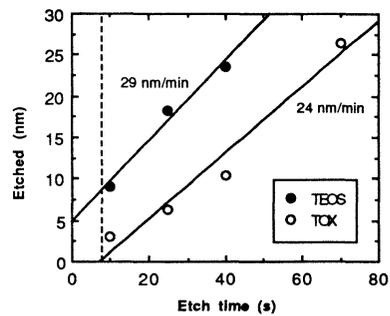
Figure 8. Etched thickness of TEOS and thermal oxide versus etch time at the saturation pressure ( $p = p_s$ ). The dotted line indicates the minimum etch time required to render a silicon wafer hydrophobic.
