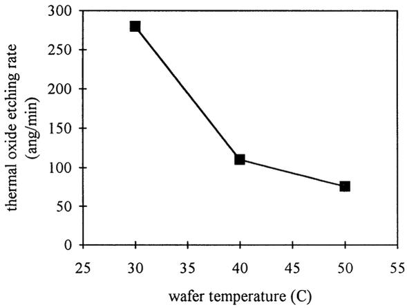
Figure 3. Dependence on wafer temperature (1000 sccm N<sub>2</sub>/IPA; 500 sccm HF; 1000 sccm N<sub>2</sub>; 100 torr).
