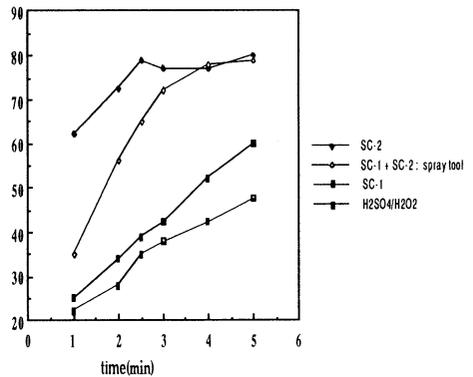
Figure 15 : Contact angle as a function of the dipping time in a 0.1 % HF solution for different chemical oxides.
