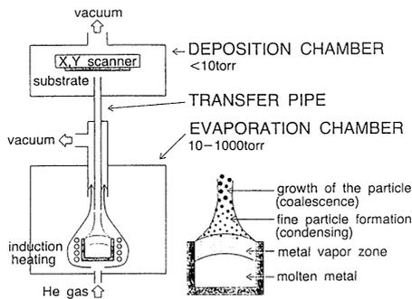
**Figure 1. Schematic diagram of the sample preparation apparatus (Gas Deposition Method).**
