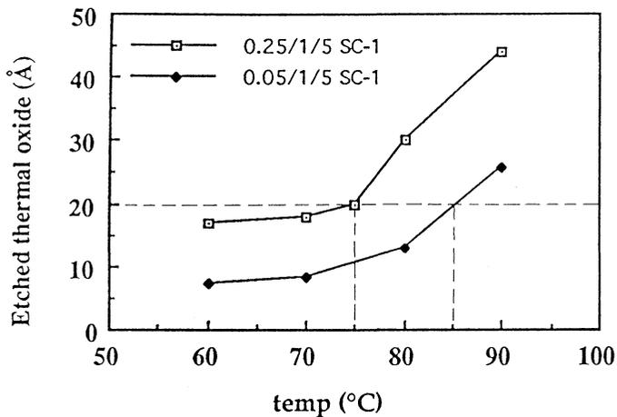
Figure 1: etched thermal oxide per 10 minutes immersion time for two different  $\text{NH}_4\text{OH}/\text{H}_2\text{O}_2/\text{H}_2\text{O}$  mixtures as a function of temperature.
