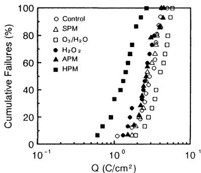
Figure 3. Cumulative failure under the negatively biased metal electrodes of MOS diodes with 6nm thick gate oxide films incorporating chemical oxides formed by various chemicals, as the current through the oxide is kept constant.
