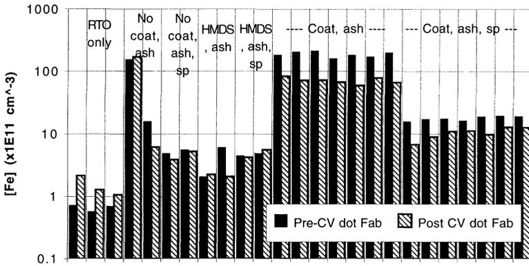
Fig. 1. Iron concentration ( $\times 10^{11} \text{cm}^{-3}$ ) versus process condition both before and after C-V dot fabrication
