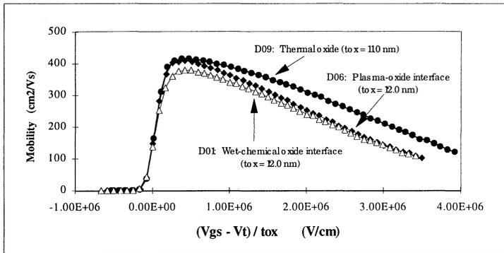
**Figure 3:** MOSFET mobility,  $\mu_{\text{eff}}$ , in the linear region ( $V_{\text{ds}} = 0.05\text{V}$ ) versus effective field,  $(V_{\text{gs}} - V_{\text{T}})/t_{\text{ox}}$ , in the gate oxide showing the detrimental effects of the wet-chemical native oxide interface.
