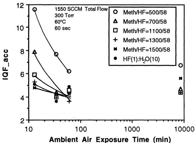
Fig. 3. IQF<sub>acc</sub> vs. time for different CH<sub>3</sub>OH flow rates.
