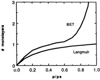
Figure 1. Langmuir and BET adsorption as a function of the relative pressure  $p/p_s$ .
