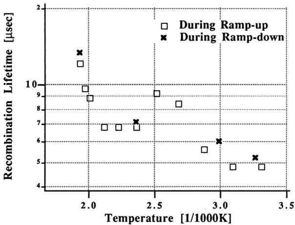
Figure 2. The photoconductivity recombination lifetime of an iron-contaminated-but-cleaned wafer as a function of temperature for both ramp-up and ramp-down.
