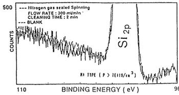
Figure 8 XPS spectrum of n<sup>+</sup> silicon wafer surface after cleaned with HF-H<sub>2</sub>O<sub>2</sub> solution (HF:0.5%, H<sub>2</sub>O<sub>2</sub>:10%) by spin method in nitrogen gas sealed process.
