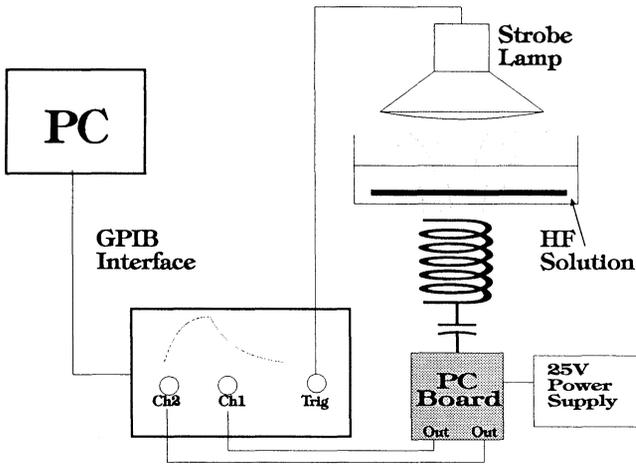
Fig. 1: Schematic of the radio-frequency photoconductive decay apparatus. The system is computer-controlled.
