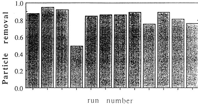
Figure 3: Particle removal efficiency ( $\phi_{LSE} > 0.5 \mu\text{m}$ ) for different runs of a  $\text{NH}_4\text{OH}/\text{H}_2\text{O}_2/\text{H}_2\text{O}$  (0.25/1/5) mixture at  $70^\circ\text{C}$ .
