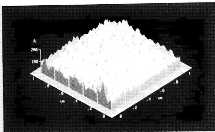
Figure 2. A representative AFM scan of H-plasma cleaned silicon at 150°C for 10 minutes with a process pressure of 15 mTorr
