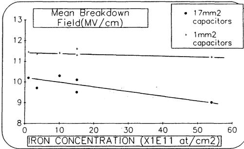
Figure 9 : Evolution of mean breakdown fields versus wafer Iron contamination present before 7 nm oxidation
