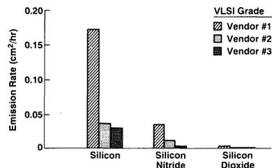
**Figure 4. Comparison of alpha-particle emission rates from three wafer-surface types and acid from three different vendors**
