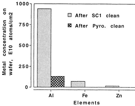
Figure 9, Removal of SC1-induced metallic contaminants by Pyrochemical cleaning.
