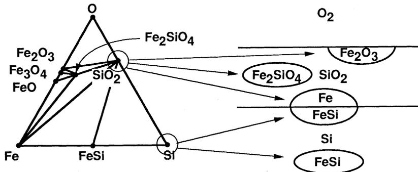
Figure 2. The phase diagram for the Fe/Si/O system is shown (other silicides neglected for clarity). The likely chemical forms of Fe in a MOS structure are shown on the right. The substrate is best represented by the lower right corner of the phase diagram in equilibrium with  $\text{SiO}_2$  and  $\text{FeSi}$ , whereas the oxide in an oxidizing ambient would be in equilibrium with  $\text{Fe}_2\text{O}_3$  and  $\text{Fe}_2\text{SiO}_4$ .
