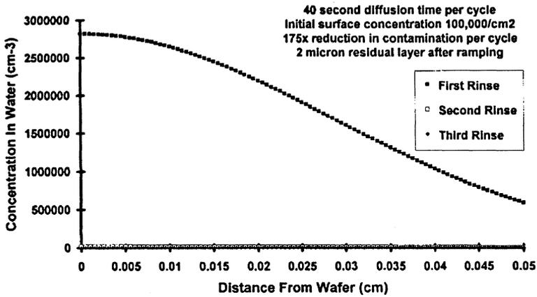
Figure 3. The calculated concentration of contaminants that have diffused away from the surface of the wafer in the rinse water for a diffusion time of 40 seconds. During a 20 second ramp at 500 rpm, all but 2  $\mu\text{m}$  of this layer would be spun off of the wafer by centrifugal force. The residual contamination in this 2  $\mu\text{m}$  layer is 0.57% of the initial surface contamination.
