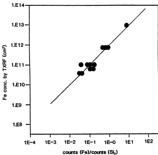
**Figure 2.** Fe surface concentration determined by TXRF versus the normalized intensity of Fe ( $\text{Fe}/\text{Si}_2$ ) determined by TOF-SIMS. The approximate analysis depth for TOF-SIMS is approx. 50 Angstroms.
