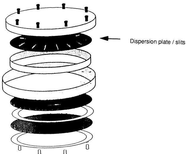
Fig. 1. Downstream oxide etcher chamber construction-exploded view.
