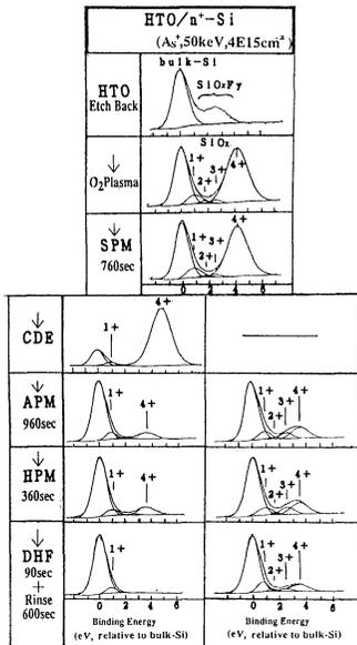
Figure 3 Si(2p) XPS spectra of  $n^+$ -Si surfaces after each treatment step.
