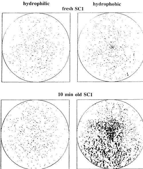
Figure 8: Light point defects (LSE:  $0.10 - 0.19 \mu\text{m}$  offzone  $5\text{mm}$ ) after treatment in a  $1 \text{ w-ppb}$  Fe spiked SC1 solution ( $0.25/1/5$  at  $70 \text{ }^\circ\text{C}$ ). The different wafers were taken out from 2 consecutively cleaned batches.
