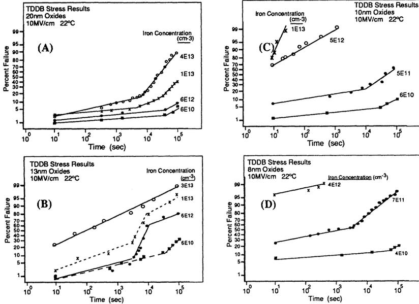
Figure 5: TDDB data for various iron concentrations and oxide thicknesses. 100 MOSDOTs were tested for each oxide thickness and iron concentration. Oxide thicknesses: (a) 20nm, (b) 13nm, (c) 10nm, (d) 8nm.
