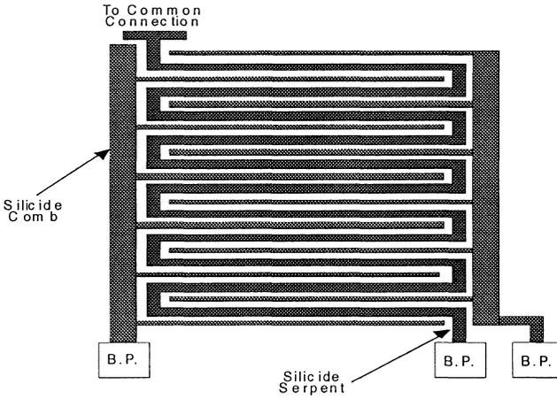
Figure 8: Serpentine and comb structure for measuring bridging and continuity.
