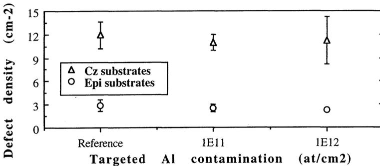
**Figure 4:** Defect density extracted from the field breakdown ( $E_{BD}$ ) yield defined at 12 MV/cm for 15 nm gate oxide capacitors fabricated on Cz and Epi substrates that have received no,  $10^{11}$  and  $10^{12}$  atoms/cm<sup>2</sup> pre-oxidation Al contamination.
