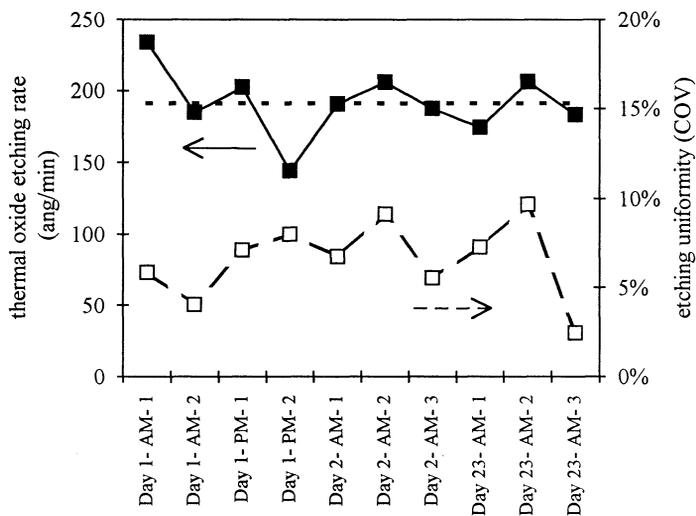
Figure 2. Etching rate repeatability and uniformity at 40 C and 100 torr.
