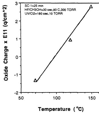
Fig. 8 Oxide charge vs. wafer temperature during UV/Cl<sub>2</sub> exposure.
