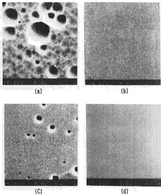
Fig.6 SEM photographs of the N type Si(100) wafer surface after immersed in (a) 630BHF (HF=6wt%, NH<sub>4</sub>F=30wt%), (b) 630BHF containing 400ppm hydrocarbon anionic surfactant, (c) BHF of low NH<sub>4</sub>F concentration (HF=6wt%, NH<sub>4</sub>F=15wt%), and (d) BHF of low NH<sub>4</sub>F containing 400ppm hydrocarbon anionic surfactant for 120 hours at 25 °C.
