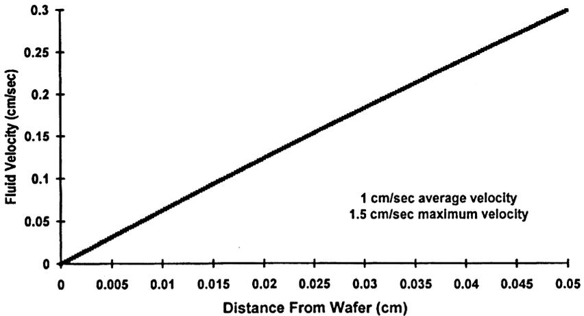
Figure 2. The fluid velocity profile near the wafer in an overflow rinse bath with an average fluid velocity of 1 cm/sec.
