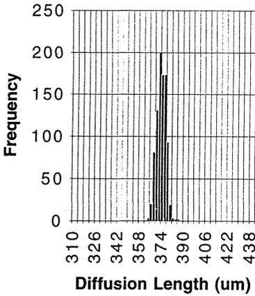
Fig. 3. L measurements of p-type wafer.  $L=374\mu\text{m}$ ,  $N=900$ ,  $\sigma=3.35\mu\text{m}$ .
