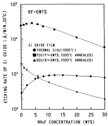
Fig.7 Relationship between the etching rate of Si oxide films and the NH<sub>4</sub>F concentration in BHF.
