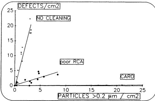
Figure 6 : Example of 7 nm dry oxide sensitivity to "natural" particles for different pre-gate cleanings
