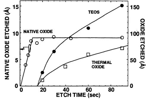
Fig. 6. Etch curves for thermal oxide, TEOS, and native oxide using anhydrous HF and IPA.
