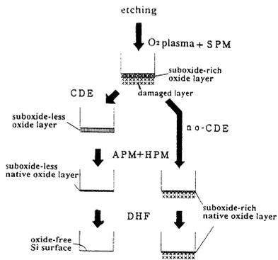
Figure 4 A model of variation of contact-hole-bottom Si surfaces through treatment processes.
