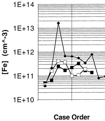
Fig. 6. [Fe] data from three older model processors. The 1E13 level shown was the result of a scratched rotor.
