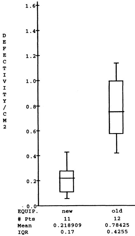
Fig.3. Snake/comb defectivity boxplot versus post planarization RIE megasonic cleaning processes using different machines.
