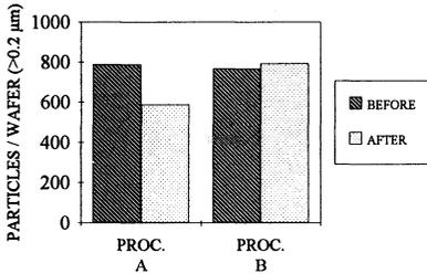
**Figure 2.** The average number of particles / wafer / cassette, before and after two different processes. Proc. A appears better at particle reduction, but this is not the truth, as revealed by fig. 3.
