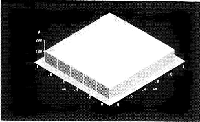
Figure 3. A representative AFM scan of H-plasma cleaned silicon at 450°C for 10 minutes with a process pressure of 15 mTorr
