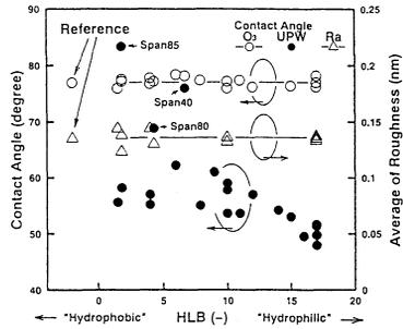
Figure 6 Cleaning efficiency of ozonized ultrapure water for organic contaminations with various hydrophobic degree
