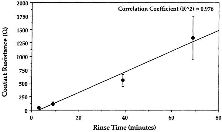
Figure 3. Contact Resistance Versus Rinse Time
