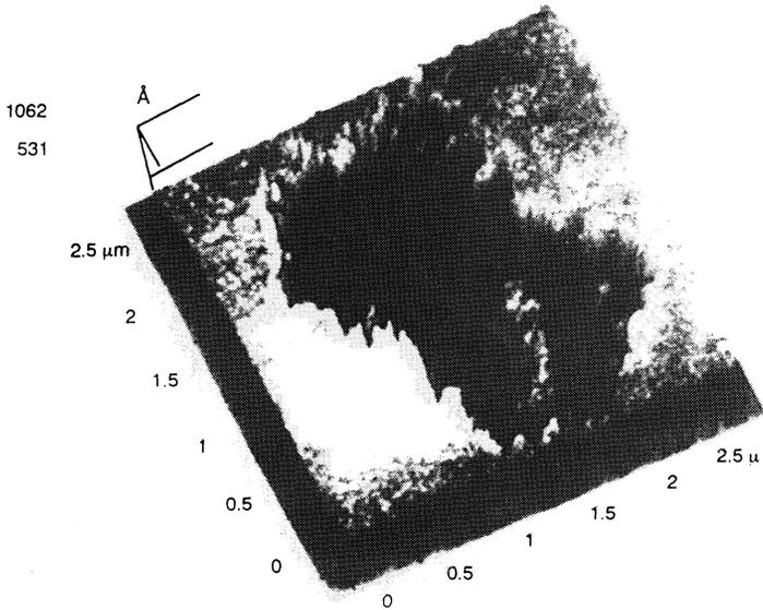
**Figure 2:** Atomic Force Micrograph of a 900Å deep pit on Si Surface of a Cu Contaminated Si wafer after 4 months in an analytical laboratory ambient.
