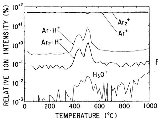
Fig. 7 APIMS-TDS spectra in argon gas related to hydrogen appeared with the forms of  $\text{ArH}^+$ ,  $\text{Ar}_2\text{H}^+$  and  $\text{H}_3\text{O}^+$ .
