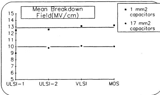
Figure 7 : Mean breakdown fields of 7 nm dry oxide obtained with the different grades of RCA cleanings
