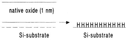
Figure 1 : Removal of the native oxide until the Si surface is passivated.
