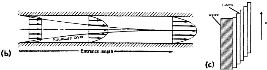
Figure 4. Wafer Gap flow field. (a) Velocity profiles, (b) Boundary layer profile, (c) Lamina shear diagram
