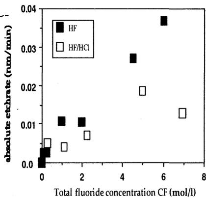
Figure 6 : Etch rates of poly-Si in HF and HF/HCl solutions as a function of the total fluoride concentration.
