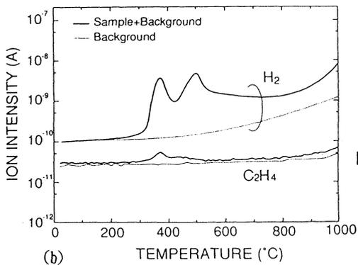
Fig. 6 Hydrogen and ethylene detected by (a) APIMS-TDS and (b) TDS.
