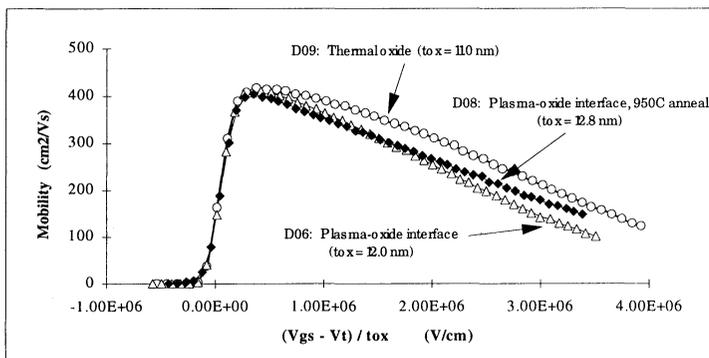
**Figure 3:** MOSFET mobility,  $\mu_{\text{eff}}$ , in the linear region ( $V_{\text{ds}} = 0.05\text{V}$ ) versus effective field,  $(V_{\text{gs}} - V_{\text{T}})/t_{\text{ox}}$ , showing the effects of a 950°C RTA of the plasma-oxide prior to RTCVD SiO<sub>2</sub>.
