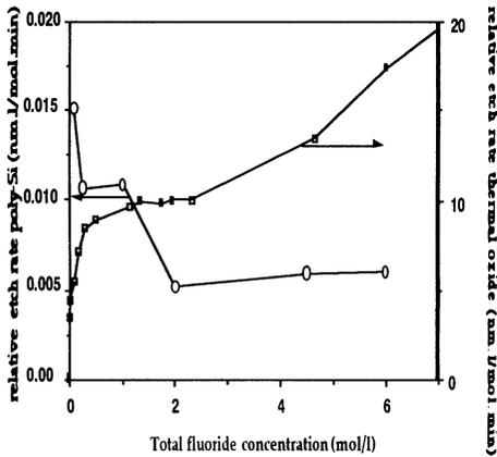
Figure 12 : Relative etch rates for thermal oxide and for poly-Si as a function of the total fluoride concentration for the HF mixture.
