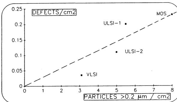
Figure 4 : Impact of particles before oxidation on pinhole generation in a 7 nm dry oxide
