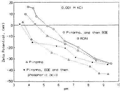
Fig. 3 Zeta potential of LPCVD nitride wafers cleaned by different methods as a function of solution pH.
