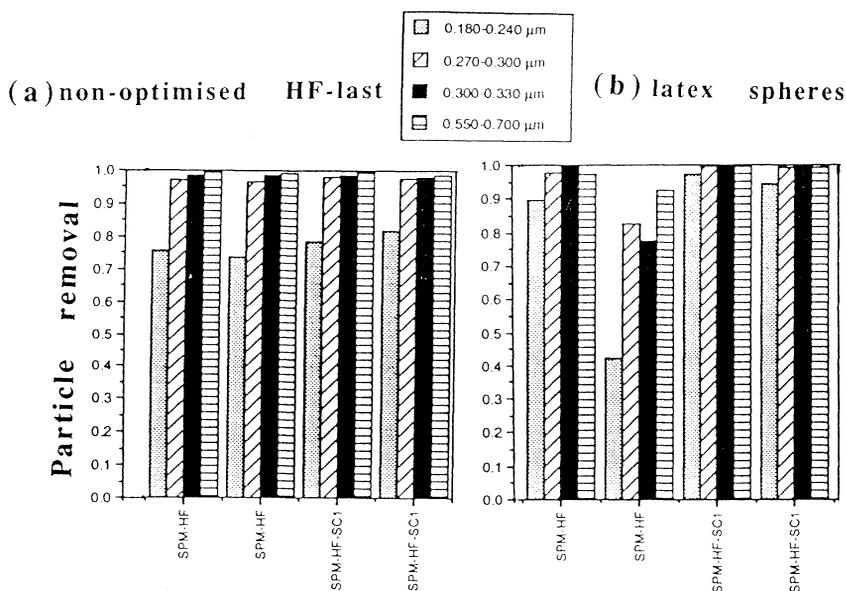
Figure 5: Particle removal efficiency of a spray processor (a) particle contamination from HF-last followed by a non-optimised drying; (b) contamination from latex spheres. SPM-HF: After the SPM-HF cycle the wafers were taken out of the tool without drying. SPM-DHF-SC1: a SC1-step was added after the SPM-DHF cycle and the conventional drying cycle was used.
