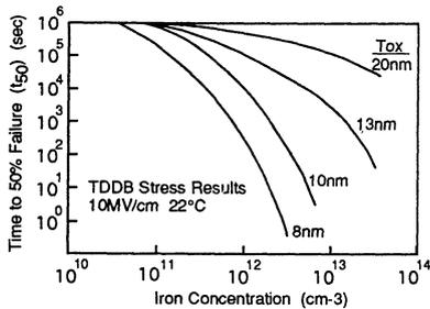
Figure 6: Time to 50% population failure ( $t_{50}$ ) versus iron concentration for various oxide thicknesses. Increased iron concentration significantly reduces the oxide wearout lifetime.
