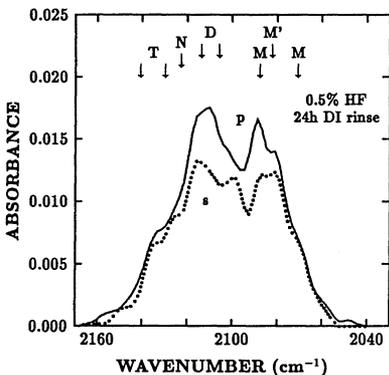
Fig. 7 : Polarized  $\text{SiH}_x$  spectra for a 24 h rinse in DI water after a 5 min etching in 0.5% $\text{HF}/\text{H}_2\text{O}$ . The increase of the monohydrides indicates (111) facetting.
