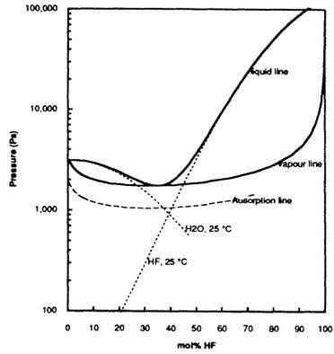
Figure 2. HF/H<sub>2</sub>O phase diagram at 25 °C. The curves are calculated based on data of Munter et al.
