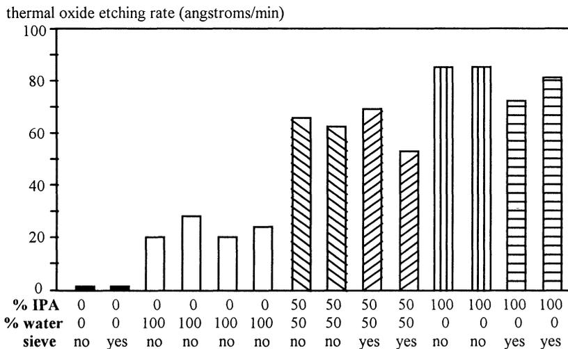
Figure 6. Dependence on added water (125 sccm through bubbler manifold; 175 sccm HF, 200 sccm N<sub>2</sub>; 40 C; 100 torr). Bar labels indicate the liquid composition in the bubbler and whether or not the gas stream through the bubbler was routed through the molecular sieve (see figure 1).
