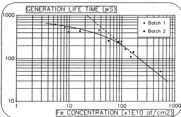
Figure 3 : Correlation between minority carriers MOS lifetime and Iron surface contamination after different SC1 baths intentionally contaminated with Iron.
