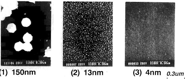
**Figure 2. SEM images of prepared sample wafers. Au ultra fine particles with diameter of 150nm to 4nm on the Si wafer are obtained by Gas Deposition Method.**
