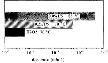
Figure 4: Decomposition rates of ultra pure SC1 mixtures: 0.05/1/5 at 85 °C and 0.25/1/5 at 70 °C compared to the ultra pure H<sub>2</sub>O<sub>2</sub> itself (metal levels: < 0.2ppb in total SC1 and < 0.4ppb in H<sub>2</sub>O<sub>2</sub>).
