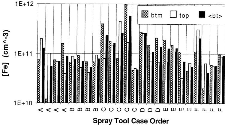
Fig. 5. Iron contamination levels obtained from various spray processors. Measurement order is indicated from left to right for each tool.
