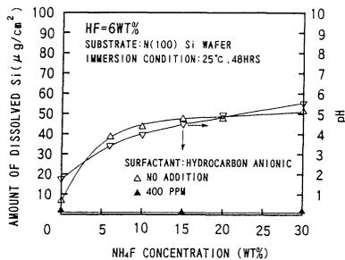
Fig.4 Dependence of pH and the amount of dissolved Si after immersed in BHF on the NH<sub>4</sub>F concentration in BHF.
