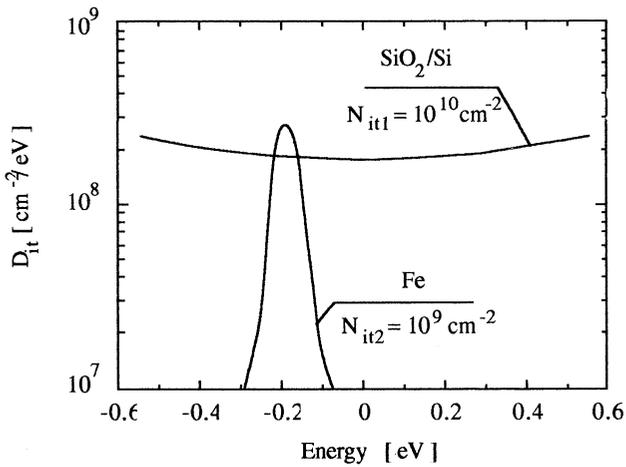
Fig. 3. Energy distribution of surface states resulting from  $\text{SiO}_2/\text{Si}$  interface (parabolic curve, donor type for negative and acceptor for positive energies, respectively) and from surface contamination by iron (gaussian curve, donor type).
