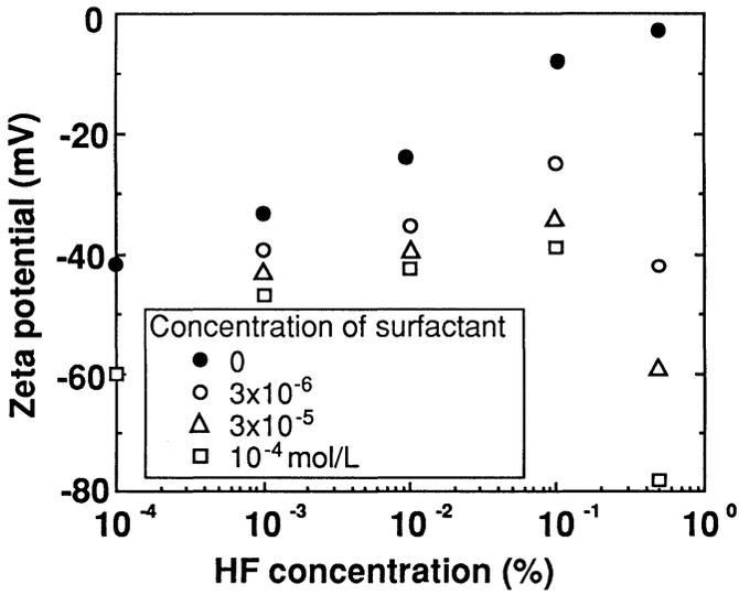
Fig. 4 Zeta potential of Si particle in HF solution
