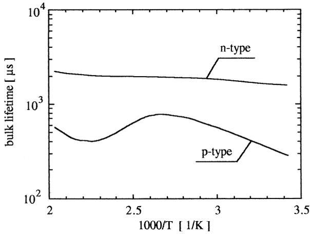
Fig. 2. Comparison of bulk recombination lifetime for n- and p-type silicon contaminated with the same amount of iron,  $N_{Fe}=5 \cdot 10^{10} \text{cm}^{-3}$ .
