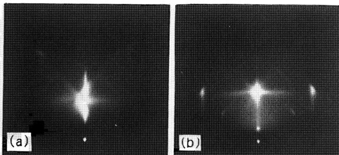
Fig. 9 RHEED pattern of (a) the silicon surface heated to  $1000^\circ C$  in argon after heating to  $650^\circ C$  in oxygen and (b) the silicon surface heated only in argon to  $1000^\circ C$ .
