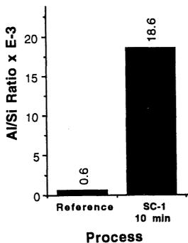
Fig. 3 SIMS results showing increased concentration of Al on the Si surface exposed to SC-1 solution.
