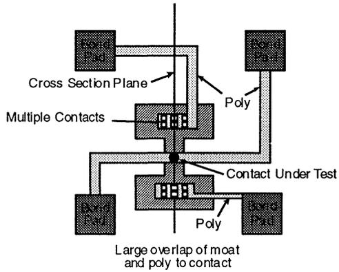
Figure 4: Van der Pauw structure for measuring single point contact resistance.
