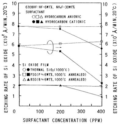
Fig.8 Relationship between the etching rate of Si oxide films and the concentration of hydrocarbon anionic and cationic surfactants in 630BHF.
