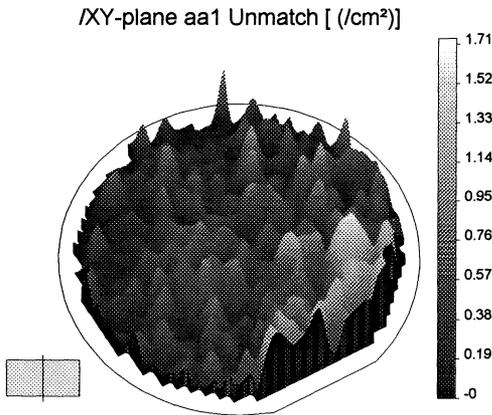
**Figure 7.** The averaged distribution of particles added to one sealed cassette of wafers by dropping the cassette from a height of one meter. The particles are fairly large and probably originate from the cassette. Their distribution is centered close to the area of impact.
