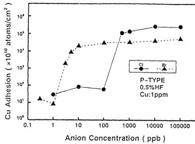
Figure 9 The relationship between the halogen concentration and the Cu adhesion onto p-type Si surface
