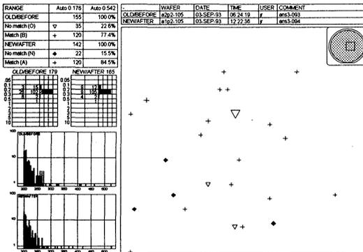
**Figure 4.** A small area of an LPD map based on two measurements, the wafer processed in between. The particles removed are shown as unfilled triangles. The fixed particles, i.e. not affected by the process step, appear as crosses. The particles added are shown as filled diamonds. The size of the symbol indicate the size of the particle.
