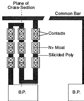
Figure 5: Contact chain structure for collecting chain resistance and yield data.
