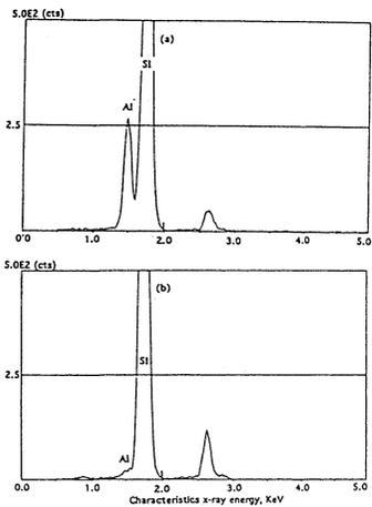
Figure 5, TXRF spectra of  $4.3E15$  atoms/cm<sup>2</sup> of Al intentionally introduced on a wafer (a) before and (b) after Pyrochemical cleaning.
