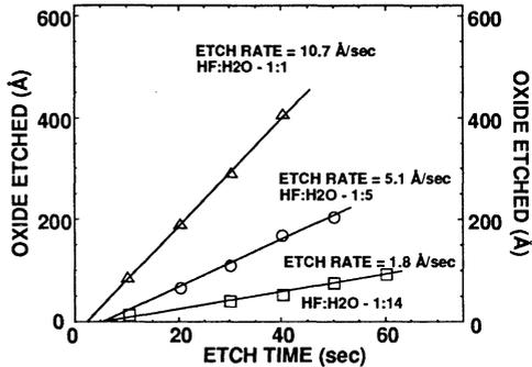
Fig. 3. The ratio of N<sub>2</sub> carrier gas flows to the azeotropic HF/H<sub>2</sub>O and H<sub>2</sub>O sources has a large affect on the thermal oxide etch rate.
