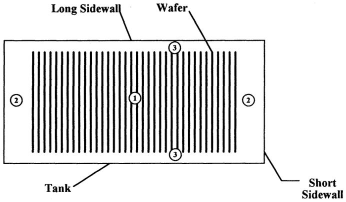
Figure 3. Rinse Tank and Wafer Geometry - Top View
