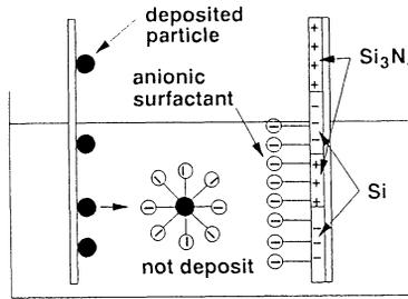
Figure 4 Proposed method to prevent particle deposition for different surfaces
