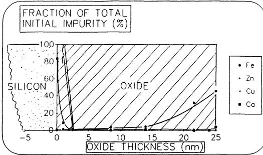
Figure 8 : Distribution of contaminants initially present at the Silicon surface after a 25 nm dry oxidation
