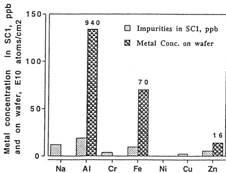
Figure 7, Metal concentration in SC1 solution and metal concentration induced on a wafer after cleaning by the SC1.
