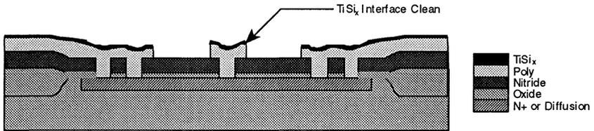
Figure 6: Cross section of polysilicon structure used for the study of pre titanium salicide cleans.
