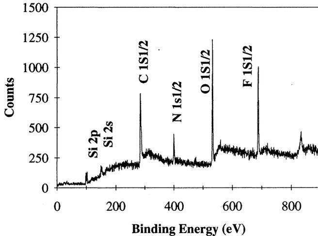
Figure 3 XPS spectrum of a sample after a  $\text{CHF}_3/\text{N}_2$  RIE.
