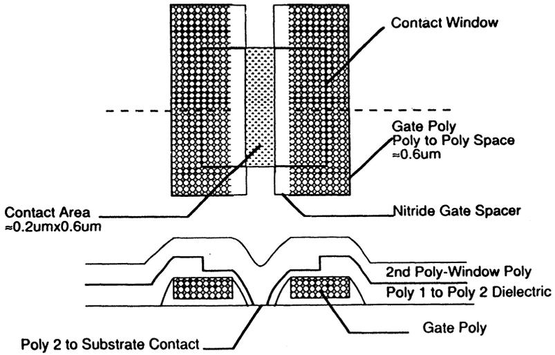
Figure 1. Self Aligned Bit Cell Contact
