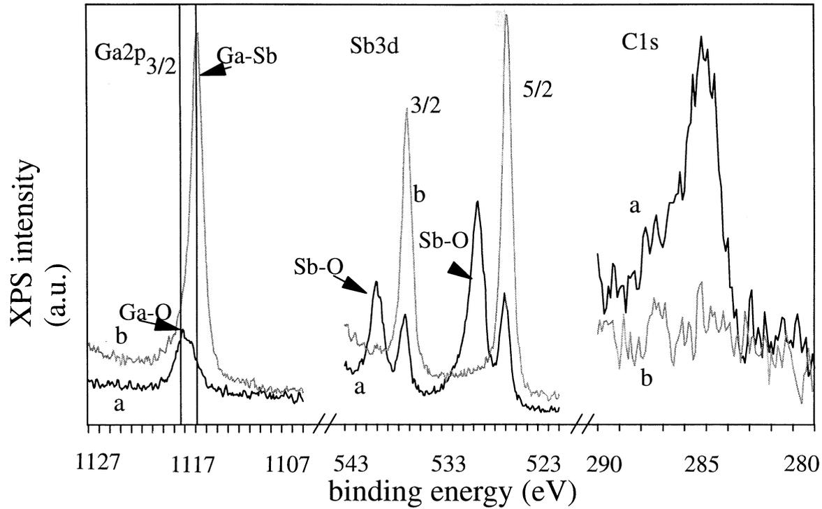
Figure 1: Processing of GaSb surfaces. a: treated 50% NH<sub>4</sub>OH b: exposed to an ECR-H at room temperature for 30 min.
