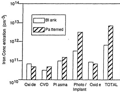
Figure 3: Fe contamination introduced by various process steps involved in LDD formation.
