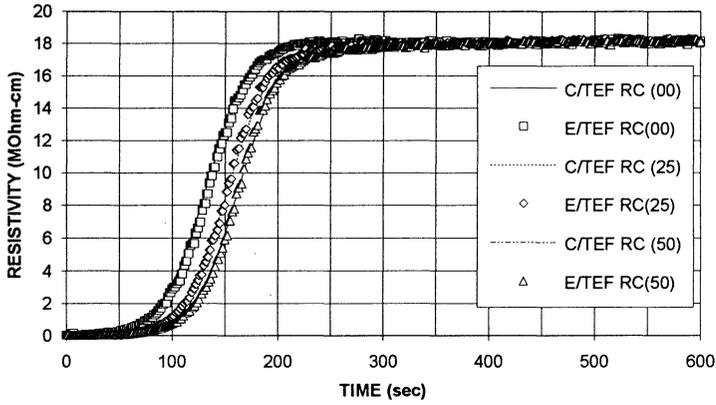
Figure 5. Experimental (points) and calculated (lines) rinse resistivity curves for the Teflon reduced cassette in the AAT with wafer load indicated in parentheses.
