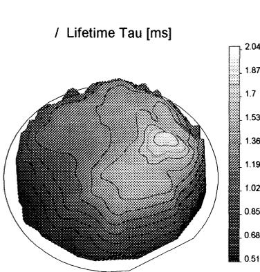
**Figure 10.** Minority carrier recombination lifetime map of a 30 Ωcm P100 wafer after dry oxidation (30 min, 900 °C). The high lifetimes recorded, almost 2 ms, indicate a very clean wafer with regard to metals.
