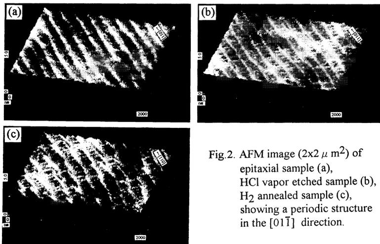
Fig.2. AFM image ( $2 \times 2 \mu\text{m}^2$ ) of epitaxial sample (a), HCl vapor etched sample (b),  $\text{H}_2$  annealed sample (c), showing a periodic structure in the  $[01\bar{1}]$  direction.
