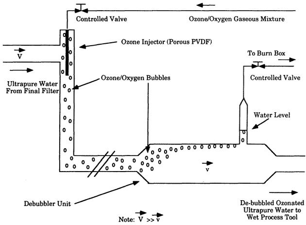
Figure 4. Ozone Injection Apparatus
