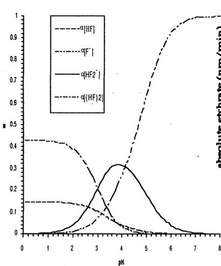
Figure 4 : Calculated composition as a function of pH for a fixed 7.5 mol/l fluoride concentration.
