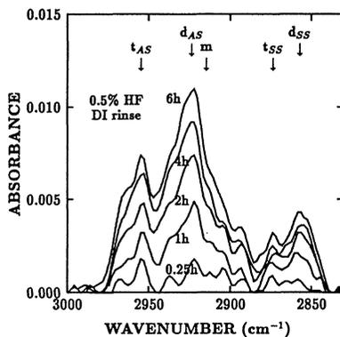
Fig. 10 : The  $\text{CH}_x$  bonds as a function of time after a H-passivation with 0.5%  $\text{HF}/\text{H}_2\text{O}$  and DI water rinse. CH (m),  $\text{CH}_2$  (d) and  $\text{CH}_3$  (t) peaks can be distinguished. Asymmetric and symmetric stretch modes are indicated by AS and SS respectively.
