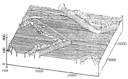
**Figure 5:** Atomic Force Microscope results from a region of 14 x 14  $\mu\text{m}^2$  of an I/I photoresist coated wafer that have been stripped for 45 min in  $\text{O}_2$  plasma and 50 min SPM solution.
