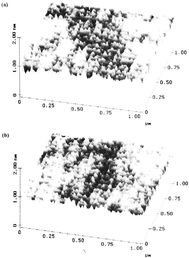
**Figure 1** The AFM image of the silicon surface exposed to hfac at 200°C (a) before and (b) after exposure. An "oxide sharpened" Digital Instruments tip was used for these measurements.
