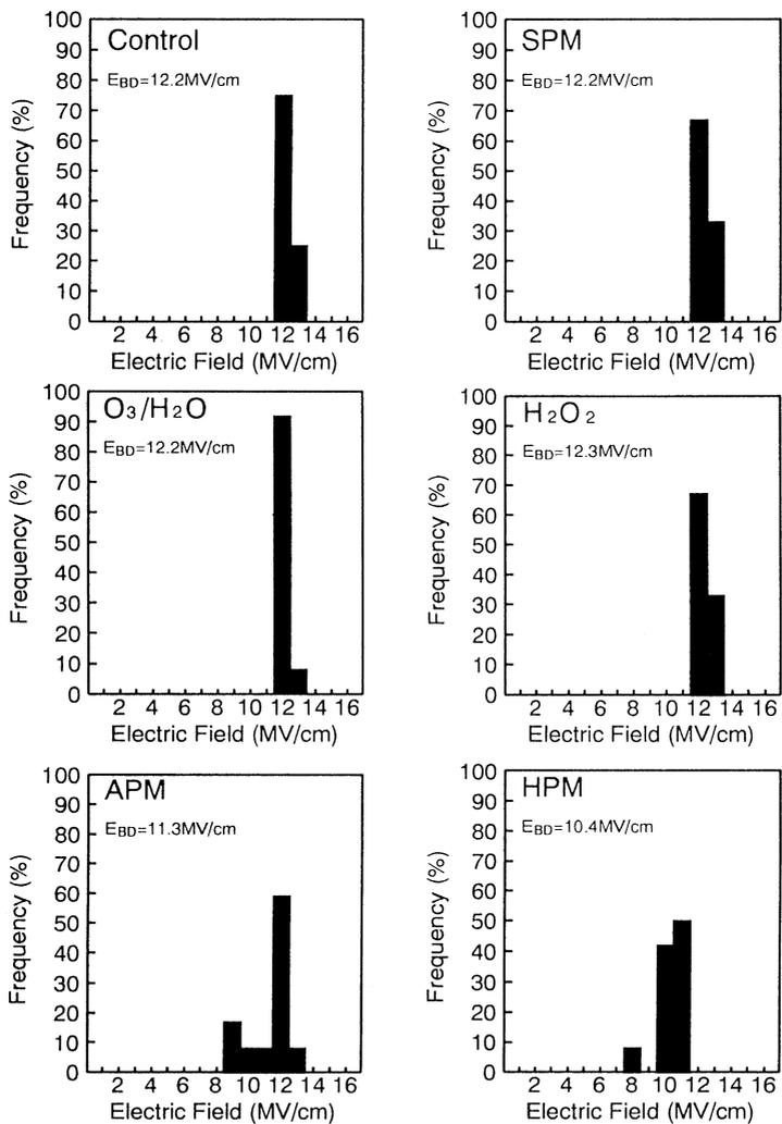
Figure 2. Dielectric breakdown characteristics of MOS diodes for 5nm thick gate oxide films incorporating chemical oxides formed by various chemicals.
