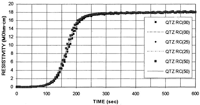
Figure 6. Experimental (points) and calculated (lines) rinse resistivity curves for the quartz reduced cassette in the AAT with wafer load indicated in parentheses.
