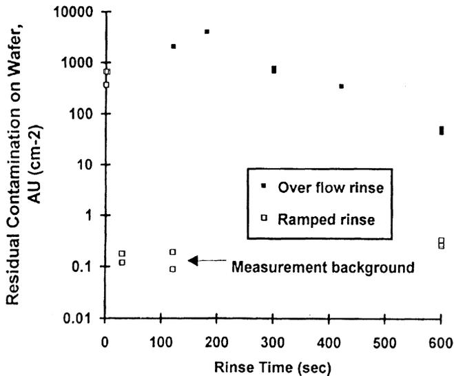
Figure 6. Experimental rinsing data for an ionic salt in an over flow rinse tank and for sodium in an acid processor utilizing ramped rinsing (5).
