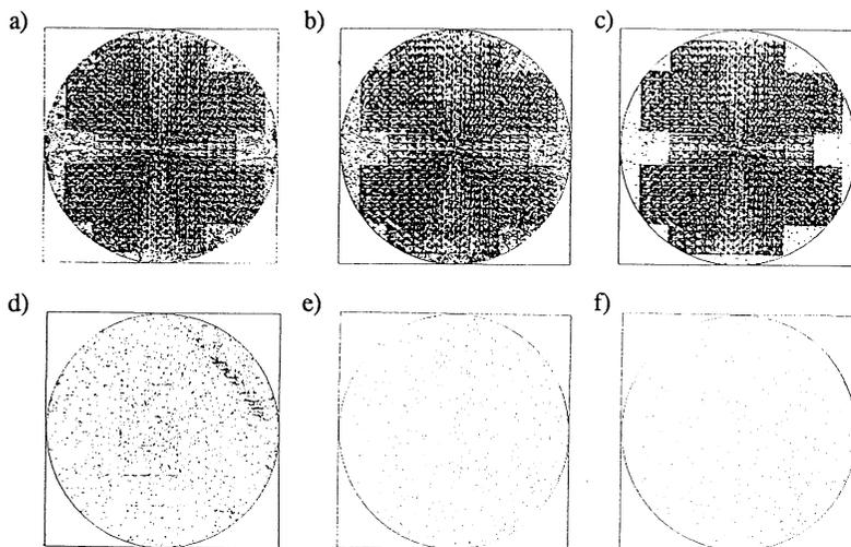
**Figure 2:** LPD plots from the Censor ANS-100: a, b and c are the results for high dose I/I photoresist; d, e and f are the results for blank photoresist. A and d show the residues after plasma dry ashing treatment; b and e indicate the effect of a further SPM wet stripping and c and f present the residues left after a final cleaning in SC1.
