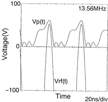
Figure 6 The waveforms of plasma potential  $V_p(t)$  and excitation electrode voltage  $V_{rf}(t)$  at 60mTorr in argon. The rf input-power is 90W.
