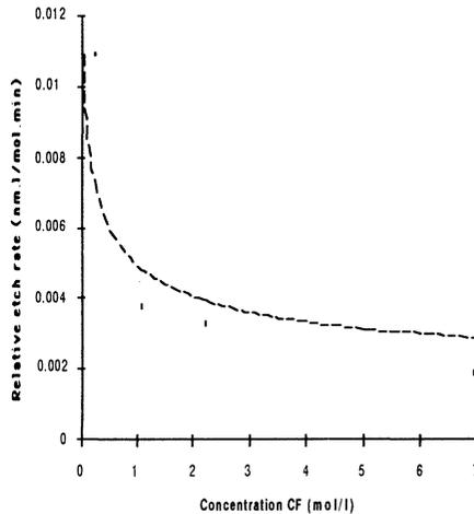
Figure 7 : Modelling of the relative etch rate of poly-Si as a function of fluoride concentration  $C_F$  in the case of a HF/HCl mixture.
