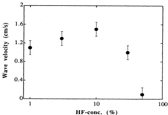
Figure 1. The contact wave velocity for room temperature, spontaneous bonding, versus the concentration of the HF etch-solution prior to bonding.
