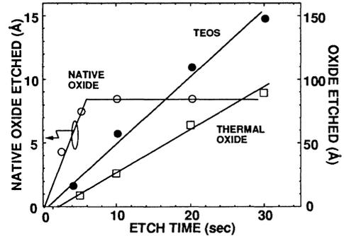
Fig. 4. Diluting the azeotropic HF/H<sub>2</sub>O source with a second H<sub>2</sub>O source improves the native oxide etch selectivity relative to TEOS and thermal oxide.
