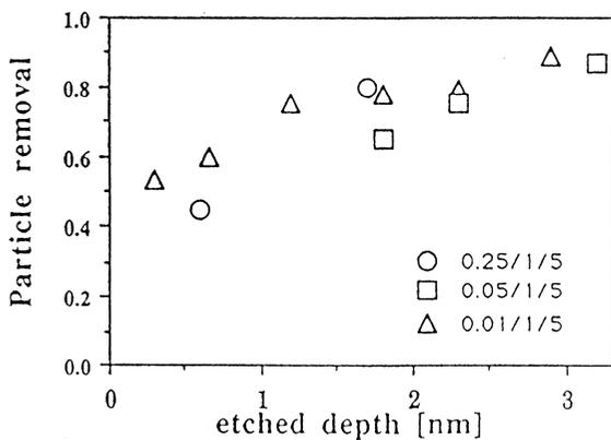
Figure 2: Particle removal efficiency ( $\phi_{\text{LSE}} > 0.5 \mu\text{m}$ ) as a function of etched thermal oxide depth for different  $\text{NH}_4\text{OH}/\text{H}_2\text{O}_2/\text{H}_2\text{O}$  mixtures at  $70^\circ\text{C}$ . Etch speed: (○) (0.25/1/5) ratio, 0.2 nm/min; (□) (0.05/1/5) ratio, 0.1 nm/min; (△) (0.01/1/5) ratio, 0.05 nm/min.
