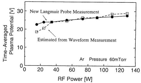
Figure 7 The rf input-power dependence of the time-averaged plasma potential which is measured by a newly developed rf Langmuir probe and estimated from the voltage waveform of the plasma excitation electrode.
