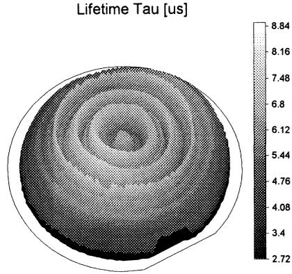
**Figure 11.** Oxygen precipitation behaviour can easily be monitored by oxidation (e.g. 4h@850 °C plus 12h@1000 °C, dry) followed by lifetime mapping. The ring structure originates from nuclei born during crystal growth.
