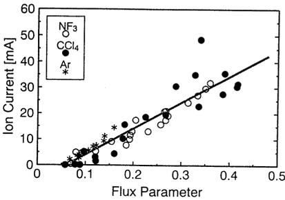
Figure 8 The relationship between the flux parameter and the ion current.
