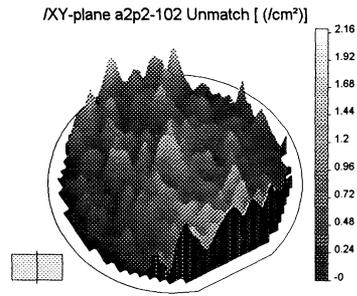
**Figure 6.** The distribution of removed particles from one cassette of wafers held stationary above a megasonic transducer.
