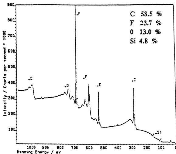
Figure 1(a). XPS results for the etched sample from the RIE reactor using  $\text{CHF}_3$  chemistry.
