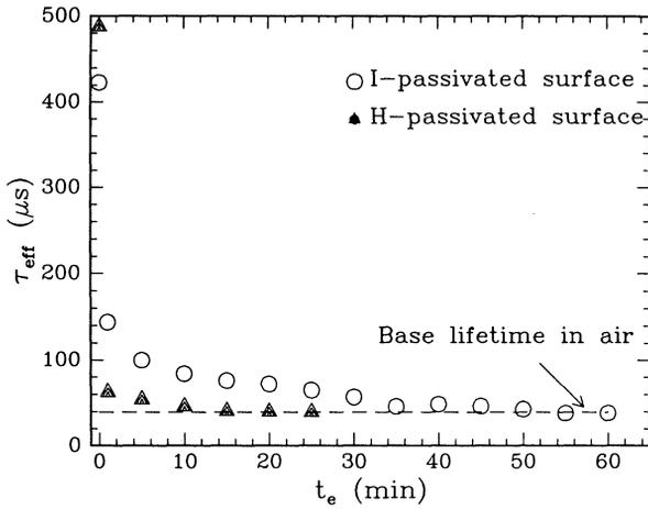
Fig. 4: Superior passivation stability of I vs. H. The wafer is float-zone n-Si(111).  $t_e$  is the time that the wafer was exposed to air.
