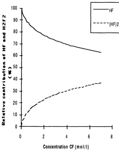
Figure 8 : Relative contributions to the etch rate of poly-Si as a function of fluoride concentration  $C_F$  in the case of a HF/HCl mixture.
