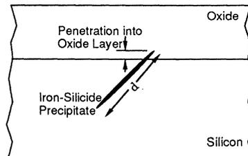
Figure 7: Oxide failure model related to iron contamination. Iron-silicide precipitates at the Si-SiO<sub>2</sub> interface cause oxide weak spots and enhanced charge injection resulting in oxide breakdown.
