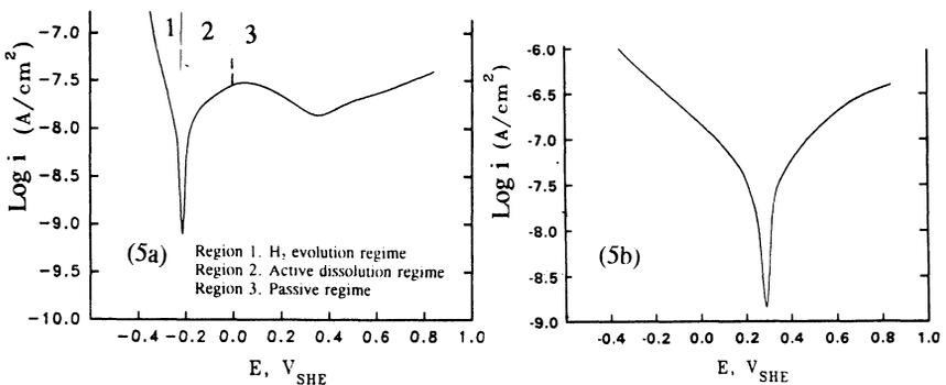
Fig. 5 Log i - E relationship for p-Si in (a) 1M HCl and (b) 25% HF
