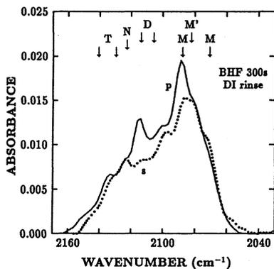
Fig. 9 : Polarized  $\text{SiH}_x$  spectrum for a 5 min etching in BHF with subsequent DI rinse.
