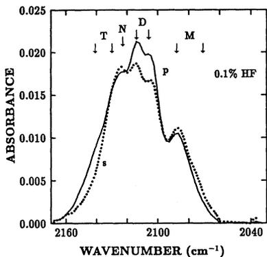
Fig. 5 : Polarized  $\text{SiH}_x$  spectrum for a 5 min etching in 0.1% $\text{HF}/\text{H}_2\text{O}$  without DI water rinsing.
