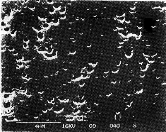
**Figure 1:** SEM of Pitted Si Surface of a Cu Contaminated Si wafer after 4 months in an analytical laboratory ambient.
