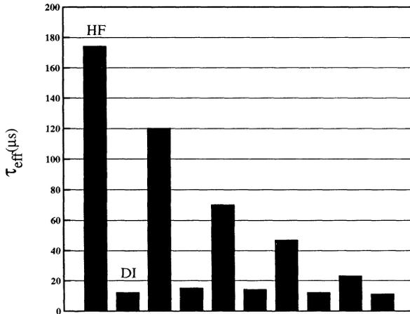
Fig. 6: Influence of sequential exposure between 48% HF and DI water on decay time for a Czochralski Si(100). The decrease in lifetime is attributed to the roughening action of DI water on Si surface. The wafer is rinsed in DI water for 5 minutes each time.
