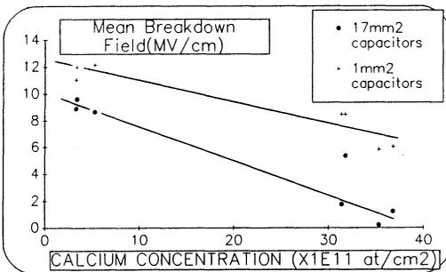
Figure 10 : Evolution of mean breakdown fields versus Calcium contamination present before 7 nm oxidation
