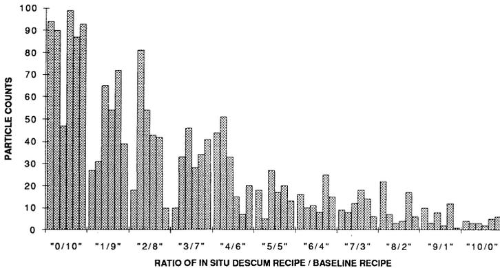
Fig. 4. Particle levels in the downstream oxide etcher due to running the *in situ* descum and baseline process at various ratios after 1250 wafers.
