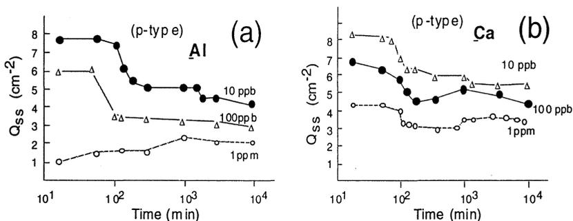
Figure 1: Surface charge as a function of exposure time to SC-1 solution contaminated with various levels of: (a) Al, (b) Ca
