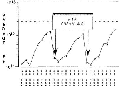
Figure 8: SPC chart of build up of heavy metals in wet sinks used for pre-oxidation cleaning, SC1-SC2. Horizontal line is upper allowable GOI contamination limit for this technology
