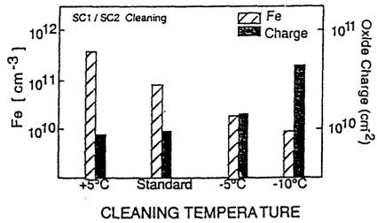
Figure 6: The effect of temperature on the SC1/SC2 cleaning. Decreasing the temperature reduces the Fe contamination, but also increases oxide charge (organic contaminants).
