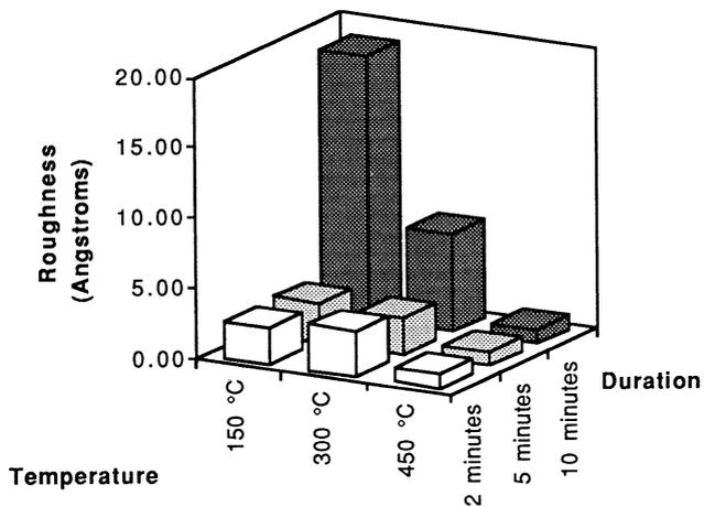
Figure 1. The relative rms roughness vs. H-plasma duration and substrate temperature. The rms roughness were obtained from 10  $\mu\text{m}$  x 10  $\mu\text{m}$  AFM scans of the surface after processing
