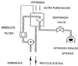
Figure 1 Advanced Chemical Distribution System
