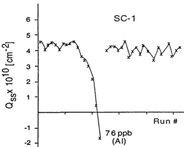
Figure 11: SPC chart of change on p-type silicon wafers measured after SC-1. Value of Al in SC-1 was measured during yield bust by ICPMS.
