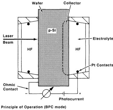
**Figure 2.** The ELYMAT measurement cell with voltage bias set to measure photo-induced current in BPC mode on a p-type silicon wafer.
