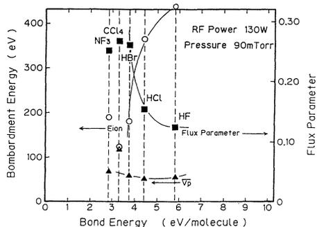
Figure 2 The relationship between bond energy and estimated plasma parameters, such as ion bombardment energy ( $E_{ion}$ ), the flux parameter and the time-averaged plasma potential ( $V_p$ ).
