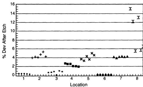
Figure 3. Etch rate data comparison of within wafer nonuniformities for 100:1 HF sink for thermal oxides from 8 different fabs.
