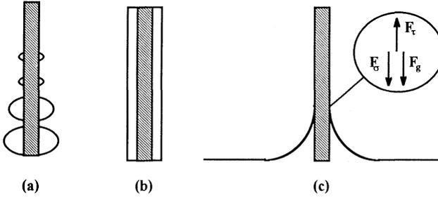
Figure 1. Physical representation of carryover volume. (a) Bulk carryover, (b) Carryover layer, (c) Force diagram
