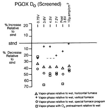
Figure 1. Upper Left. Bar graph summary of TXRF data evaluation of the relative effectiveness of vapor-phase HF with and without HCl in removing ashed photoresist transition metal residues from blanket-coated, bare silicon wafer surfaces.
