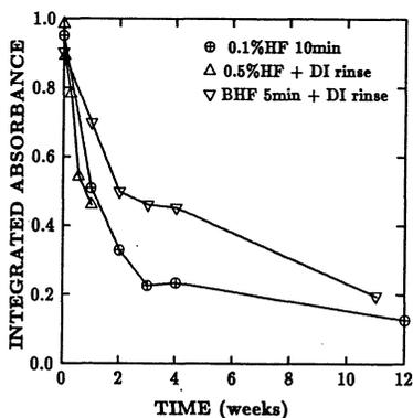
Fig. 11 : Decrease of the integrated  $\text{SiH}_x$  absorbance for different etchings when the samples are kept in cleanroom air for several weeks.
