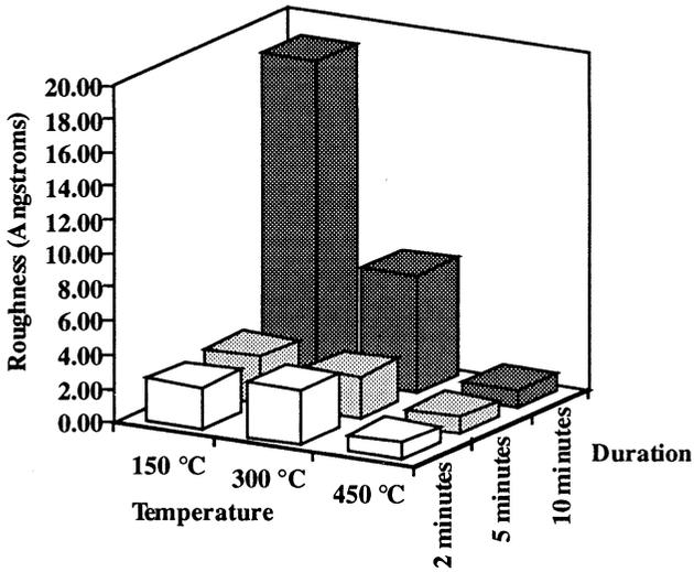
Fig. 2 Summary of the temperature and exposure time dependence of the rms surface roughness, calculated from AFM images, following H-plasma exposure.
