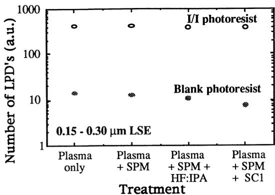
**Figure 3:** LPD's in the range of 0.15 to 0.30  $\mu\text{m}$  LSE measured on silicon wafers after a dry stripping in  $\text{O}_2$  plasma followed by a wet stripping in SPM and a final cleaning in SC1 at 70  $^\circ\text{C}$  or in 0.5%HF:0.1%IPA. (○) high dose I/I photoresist and (●) blank photoresist.
