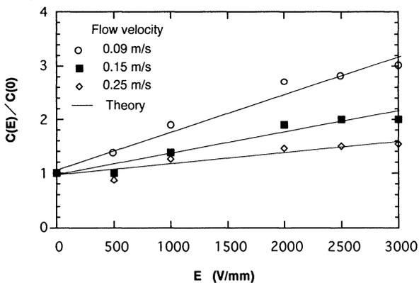
Fig. 4 Counting rates as a function of the electric field
