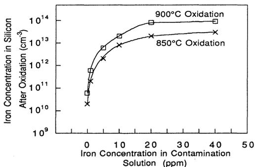
Figure 1: Iron contamination in silicon wafer resulting from spin-application of iron contaminated solution. At high solution contamination levels the wafer concentration saturates at the iron solubility level for the given oxidation temperature.
