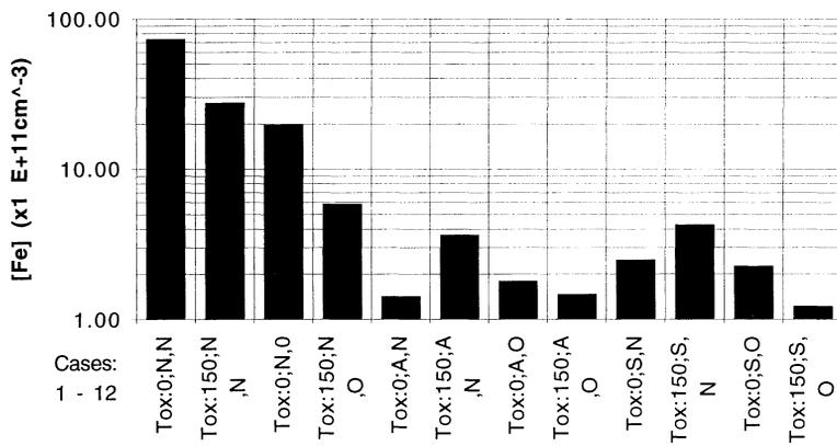
Fig. 3. Iron concentration ( $\times 10^{11} \text{cm}^{-3}$ ) versus process case. Fields are:  $T_{\text{ox}}$ : 0Å or 150Å ; Clean: N=no, A=RCA(A), S=SP ; RTA Ambient: O=O<sub>2</sub>, N=N<sub>2</sub>.
