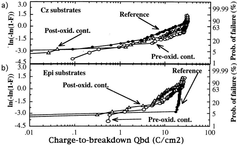
**Figure 5:** Charge-to-breakdown ( $Q_{BD}$ ) plots obtained with a current density of  $0.1\text{A}/\text{cm}^2$  for  $15\text{ nm}$  gate oxide capacitors that have received Na contamination. The results of ( $\bullet$ ) reference, ( $\circ$ ) pre-oxidation and ( $\Delta$ ) post-oxidation contaminated samples are shown for (a) Cz and (b) Epi substrates.
