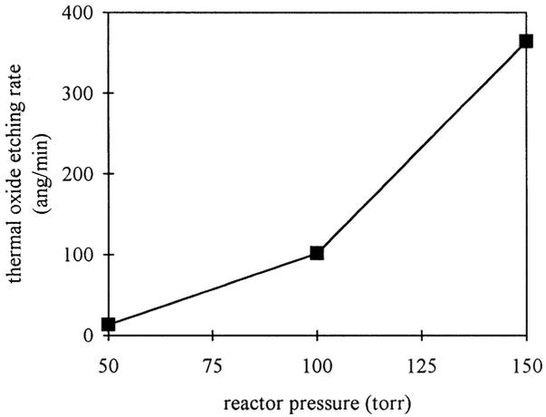
Figure 4. Dependence on pressure (500 sccm N<sub>2</sub>/IPA; 250 sccm HF, 500 sccm N<sub>2</sub>; 40 C).
