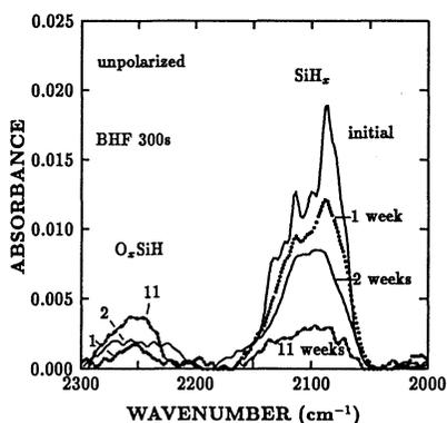
Fig. 12 :  $\text{SiH}_x$  and  $\text{O}_x\text{SiH}$  peaks as a function of storage time in air after a BHF 300s etching and subsequent rinsing in DI water.
