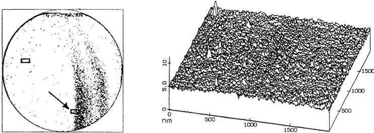
Figure 6: Decomposition-LPDs and their atomic nature: a) Light point defects (LSE: 0.15 - 0.30  $\mu\text{m}$ , offzone 0mm) after treatment in an ultra clean SC1 solution (metal levels: < 0.2ppb); typical patterns when decomposition of H<sub>2</sub>O<sub>2</sub> occurs at the PFA carrier, b) AFM plot from the roughened area of this wafer (arrow).
