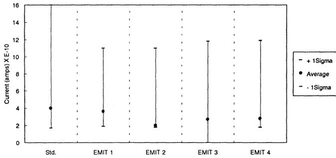
Figure 10: Junction leakage data from lot 1151.
