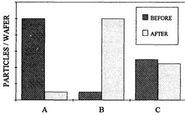
**Figure 1.** Three different cases (A, B, C) showing how processing can affect the number of particles on wafers.
