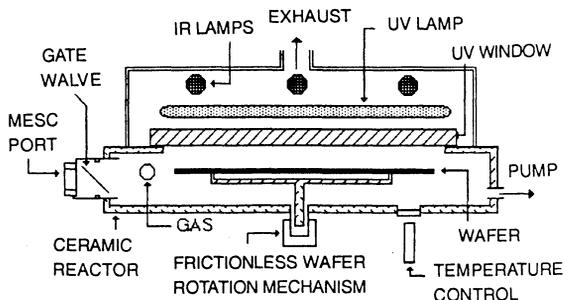
Figure 1 Schematic of the prototype cluster tool used in this study. The system also has an ozone generator not shown in this figure.
