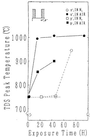
Figure 6 Temperature change of TDS peaks as a function of the exposure time periods to clean-room air and  $N_2$ .
