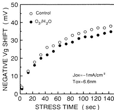
Figure 6 Gate voltage( $V_g$ ) shift of MOS diodes with 6.6nm thick gate oxide films, as the current through the oxide is kept constant.
