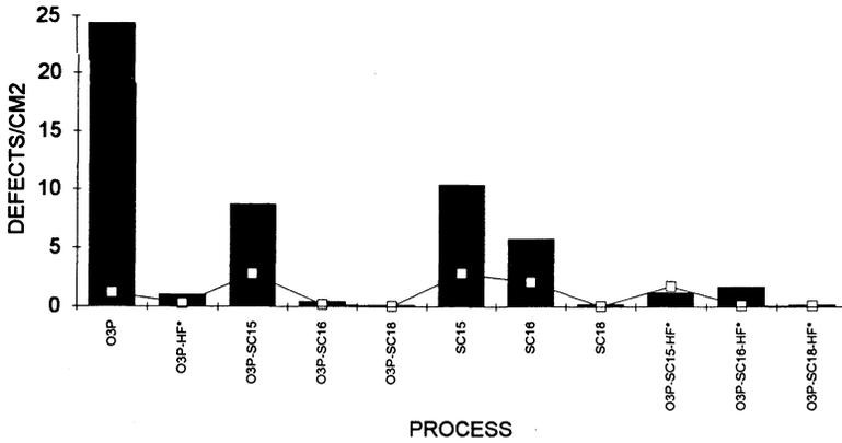
Figure 2. Defect density analysis of wet process sequences evaluated for ion implanted samples
