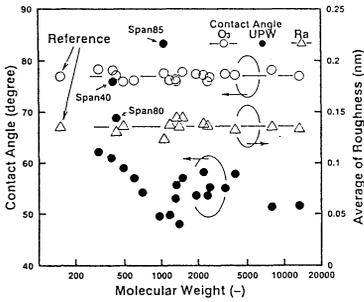
Figure 5 Cleaning efficiency of ozonized ultrapure water for organic contaminations with various molecular weight
