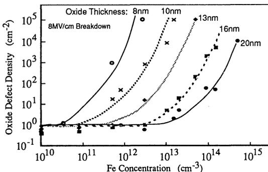
Figure 4: MOSDOT capacitor data. Oxide defect density versus iron contamination level. A defect is defined as breakdown occurring at less than 8MV/cm during ramp voltage I/V test.
