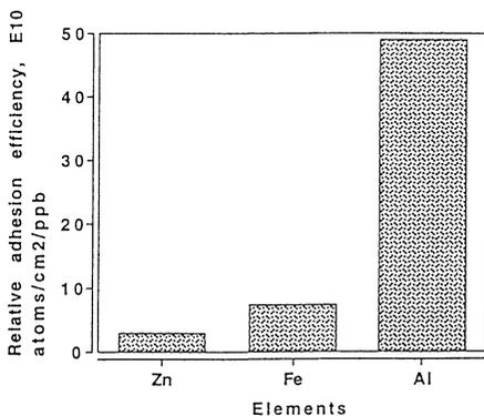
Figure 8, Relative adhesion efficiency of Zn, Fe and Al in SC1 solution.
