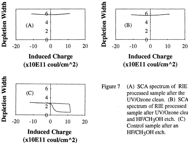
Figure 7 (A) SCA spectrum of RIE processed sample after the UV/Ozone clean. (B) SCA spectrum of RIE processed sample after UV/Ozone cleaning and HF/CH<sub>3</sub>OH etch. (C) Control sample after an HF/CH<sub>3</sub>OH etch.
