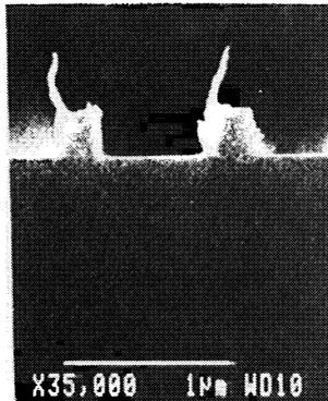
3. Polymer residue seen after polysilicon etch. Piranha - vapor HF - piranha clean sequence efficiently removes this.
