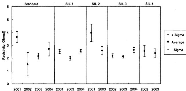
Figure 16: Sheet resistivity data titanium salicide polysilicon for lots 2001 - 2004.
