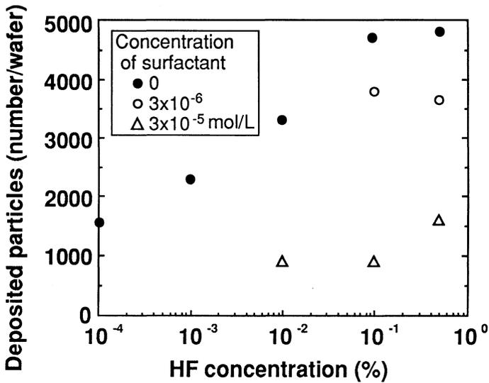
Fig.5 Particle deposition in HF solution
