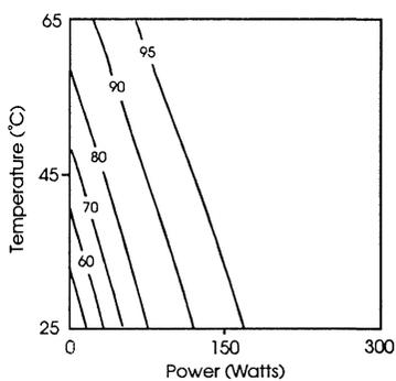
**Figure 2.** Contour plot of cleaning efficiency as a function of megasonic power and bath temperature with  $[\text{NH}_4\text{OH}]/[\text{H}_2\text{O}_2] = 0.10$
