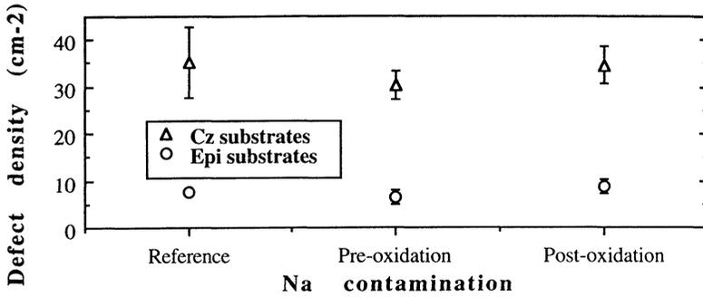
**Figure 2:** Defect density extracted from the field breakdown ( $E_{BD}$ ) yield defined at 12 MV/cm for 15 nm gate oxide capacitors fabricated on Cz and Epi substrates that have received no, pre and post oxidation Na contamination.
