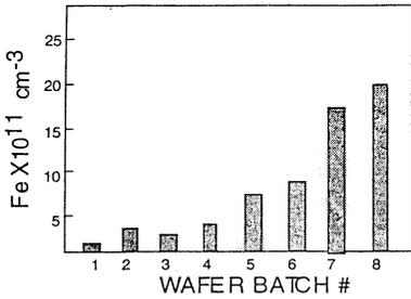
Figure 7: Build-up of heavy metals in cleaning sinks (SC1-SC2) as a function of cleaning cycles. (Chemicals not replaced)
