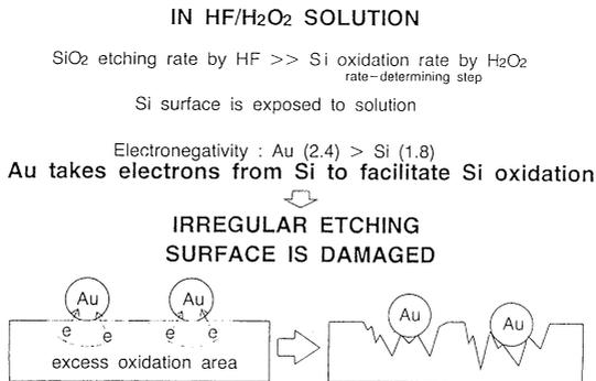
**Figure 9. Mechanism of surface microroughness caused by Au particles with DHF-H<sub>2</sub>O<sub>2</sub> cleaning.**
