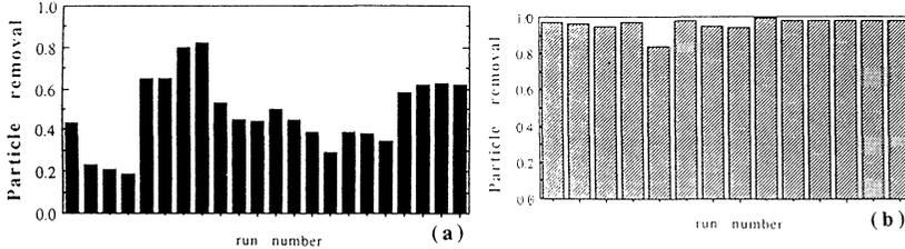
Figure 4: Particle removal efficiency ( $\phi_{LSE} > 0.5 \mu\text{m}$ ) for different runs of a spray processor (a) RCA-clean (SC1-SC2), (b) SPM-DHF-SC1-SC2 cycle
