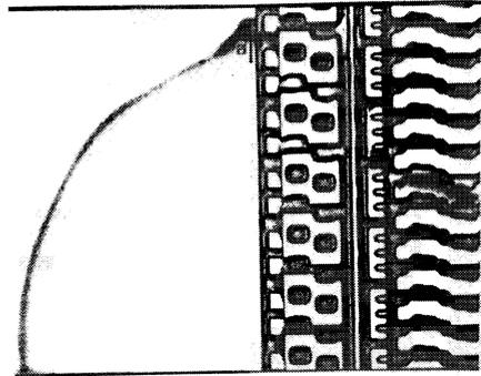
2. Liquid residue defects seen on patterned wafers. Residue is probably a fluosilicic acid polymer.
