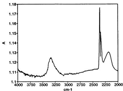
Fig. 2 FTIR spectrum of PECVD silicon nitride film.
