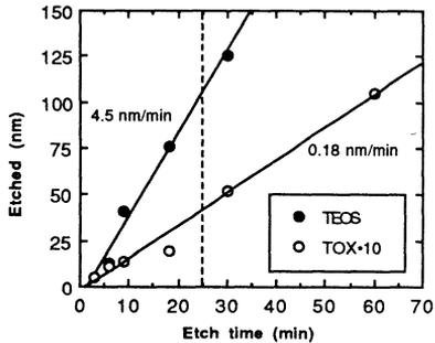
Figure 4. Gas phase etching of different oxides. The amount of etched thermal oxide (TOX) and TEOS oxide as a function of the etch time. The dotted line indicates the minimum etch time required to render a silicon wafer hydrophobic.
