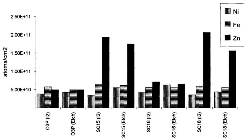
Figure 4. Surface contamination analysis using TRXRF for O3P versus heated SC1 processes
