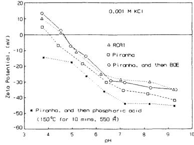
Fig. 4 Zeta potential of PECVD nitride wafers processed in various cleaning solutions as a function of pH.
