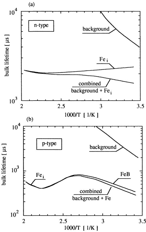
Fig. 1. Theoretical temperature dependence of bulk recombination lifetime for (a) n-type and (b) p-type silicon contaminated with iron. An additional lifetime reduction due to an unknown background contamination is also shown.
