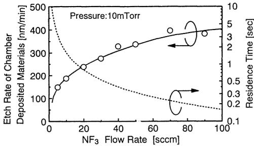
Figure 4 The etch rate of a mixture of photoresist and an OCD silica solution modeled sub-products of etching chamber and the gas residence time as a function of  $\text{NF}_3$  gas flow rate at a constant pressure of 10mTorr.
