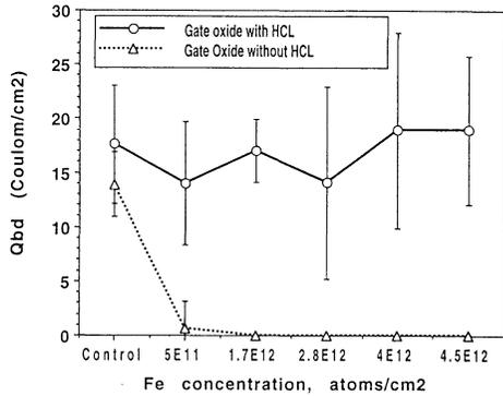
Figure 4. Effect of HCl during oxidation on gate oxide integrity.
