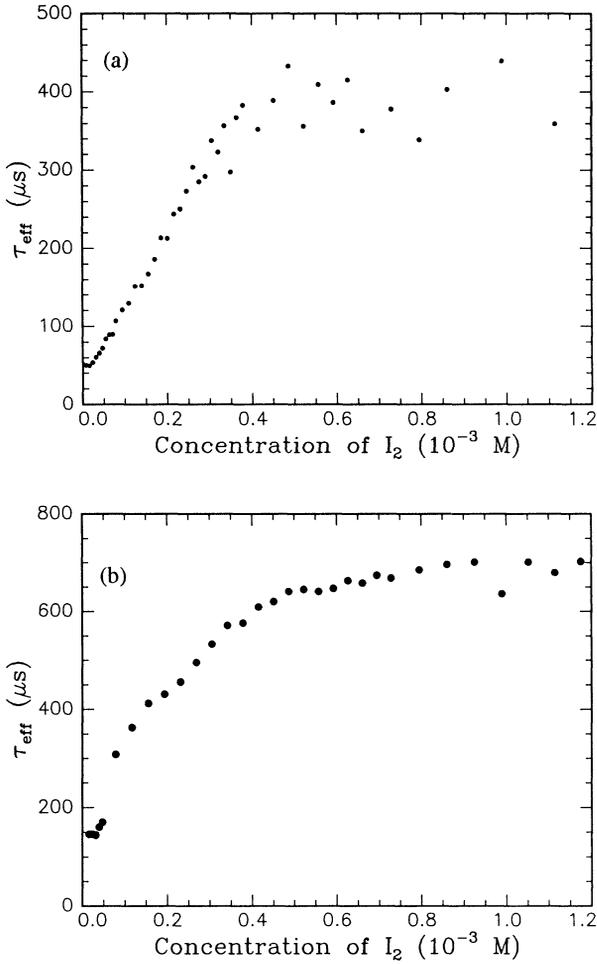
Fig. 3: The variation of lifetime with iodine concentration in methanol. The increase in lifetime is attributed to the passivation of the silicon surface with iodine. The surface recombination velocity is lowered as iodine bonds to the surface atoms. (a) n-type FZ Si(111) in non  $\text{N}_2$ -bubbled methanol and (b) p-type FZ-Si in  $\text{N}_2$ -bubbled methanol.
