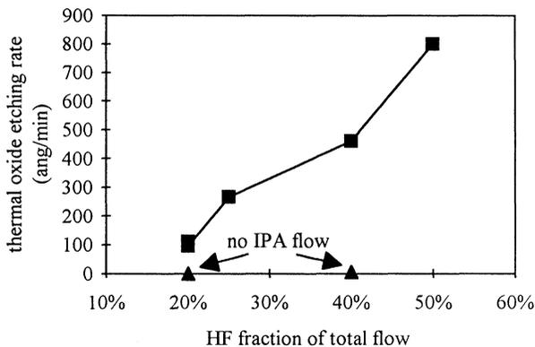
Figure 5. Dependence on HF fraction (1000 sccm N<sub>2</sub>/IPA; 2000-2500 sccm total flow; 40 C; 100 torr).
