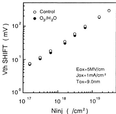
Figure 5 Threshold voltage( $V_{th}$ ) shift of n-MOSFET with 9nm thick gate oxides as a function of the number of injected electrons.
