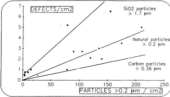
Figure 5 : Example of relationship between the nature of particles before oxidation and pinholes obtained on a 7 nm dry oxide
