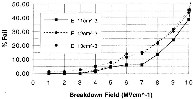
Fig. 2. Oxide breakdown percent failure, by average iron contamination level, versus oxide field. Field axis indicates bins for comparison between [Fe].
