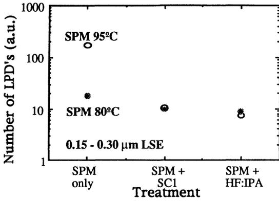
**Figure 6:** LPD's measured in the range of 0.15 to 0.30  $\mu\text{m}$  LSE on silicon wafers coated with blank photoresist after stripping for 10 min in SPM at 95  $^{\circ}\text{C}$  (o) or 80  $^{\circ}\text{C}$  (•) and further cleaned for 20 min in SC1 at 70  $^{\circ}\text{C}$ . or for 2 min in 0.5%:0.1% HF:IPA.
