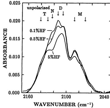
Fig. 4 : Unpolarized spectra after etching with a 0.1%, 0.5% and 5%  $\text{HF}/\text{H}_2\text{O}$  solution without DI water rinsing.
