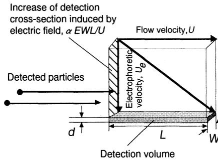
Fig. 2 Detection cross-section under the electric field
