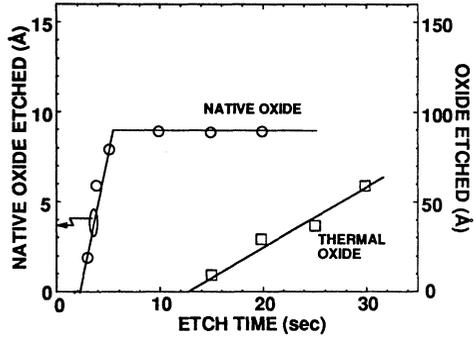
Fig. 5. Diluting the azeotropic HF/H<sub>2</sub>O with azeotropic HF/HCl increases the delay time of thermal oxide and allows selective removal of native oxide.
