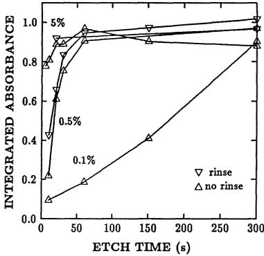
Fig. 3 : Integrated absorbance of the  $\text{SiH}_x$  stretching mode as a function of the etch time in different  $\text{HF}/\text{H}_2\text{O}$  solutions with and without rinsing.
