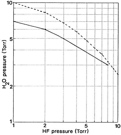
Fig. 2: Transition curve (solid line) separating controlled etch rates (nm/min) from very fast etch rates (>100 nm/min). The condensation curve as calculated by Helms and Deal (4) is also indicated (dashed line).
