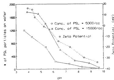
Fig. 6 Correlation between zeta potential values and extent of PSL contamination on LPCVD nitride wafers cleaned by piranha, followed by BOE.
