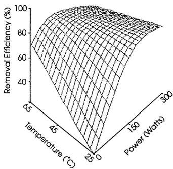
**Figure 4.** Three-dimensional response surface plot.  $[\text{NH}_4\text{OH}]/[\text{H}_2\text{O}_2] = 0.01$
