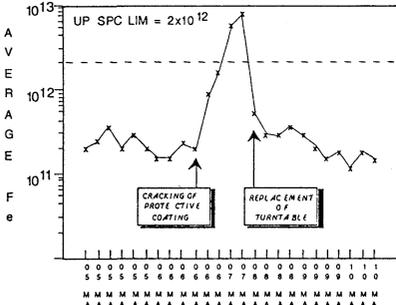
Figure 9: SPC chart for self-contained spray processor. Horizontal line is upper allowable GOI contamination limit for this technology.
