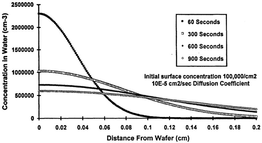
Figure 1. The calculated concentration distribution of molecular contaminants that have diffused away from the surface of the wafer into the rinse water for diffusion times of 60, 300, 600 and 900 seconds. The calculation assumes a stagnant bath and a diffusion coefficient of  $10^{-5}$  cm<sup>2</sup>/sec, typical of ionic and molecular species (4).
