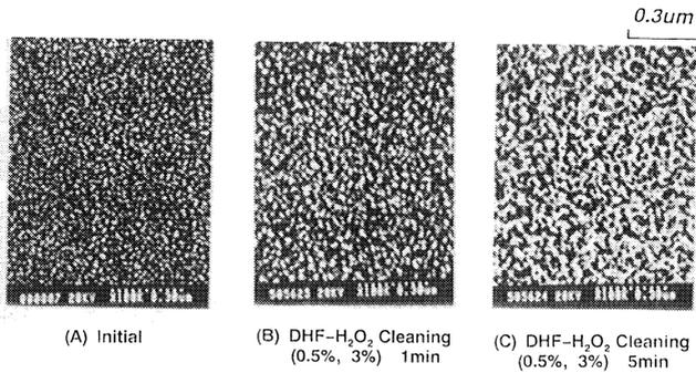
**Figure 7. SEM images of the sample wafer with Au ultra fine particles after DHF-H<sub>2</sub>O<sub>2</sub> cleaning. The Si surface got rougher.**
