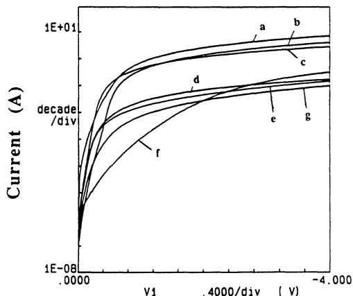
Figure I. Forward bias current for the (a) control, (b) SF<sub>6</sub>/O<sub>2</sub>, (c) CF<sub>4</sub>, (d) ISO, (e) ICP, (f) SF<sub>6</sub>/Ar, and (g) etched samples.
