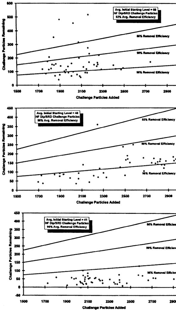
Figures 3a - 3c. Particle removal performance for treatments 1, 2 and 3. The x axis indicates the number of “HF Last” challenge particles added to the wafer over and above the count on the precleaned wafer. The y axis indicates the number of these added challenge particles remaining after the clean. Diagonal lines mark the boundaries of 85, 90 and 95% challenge particle removal efficiencies.
