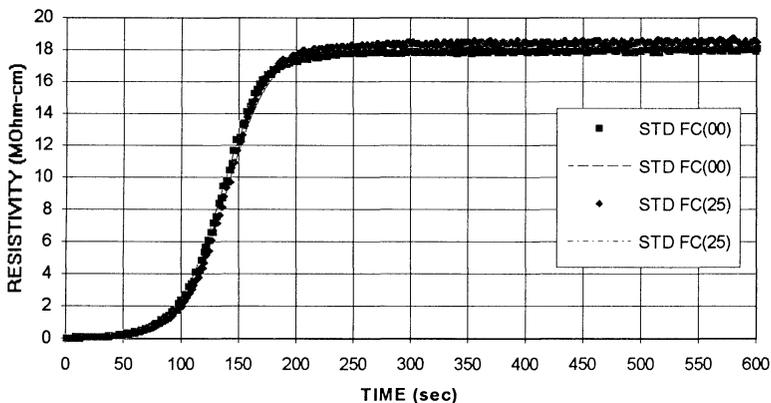
Figure 7. Experimental (points) and calculated (lines) rinse resistivity curves for the standard full cassette in the AAT with wafer load indicated in parentheses.
