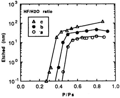
Figure 5. Etched thickness of thermal oxide as a function of the relative pressure ( $p/p_s$ ) for various HF/H<sub>2</sub>O vapour pressures.
