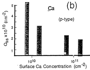
Figure 2: Surface charge measured on p-type wafers correlated to AAS measurements of: (a) surface Al concentration, and (b) surface Ca concentration
