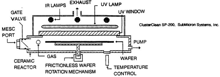
Fig. 1. Prototype commercial clusterable cleaning reactor used in this study.
