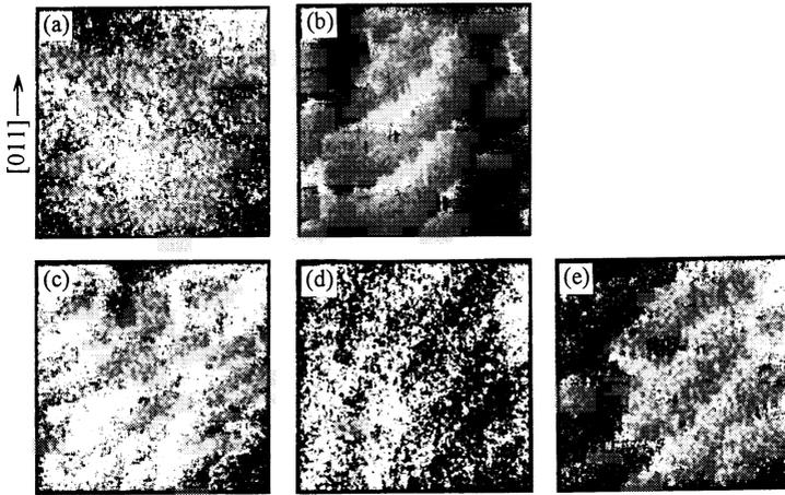
Fig. 7. AFM image ( $4 \times 4 \mu\text{m}^2$ ) of (a) mirror polished sample, (b)  $\text{H}_2$  annealed sample and  $\text{H}_2$  annealed samples after SC-1 cleaning with  $\text{NH}_4\text{OH}/\text{H}_2\text{O}_2/\text{H}_2\text{O}$  mixing ratio of (c) 1/1/5(10nm) : sample A, (d) 1/1/5(40nm) : sample B and (e) 1/10/100(10nm) : sample C.
