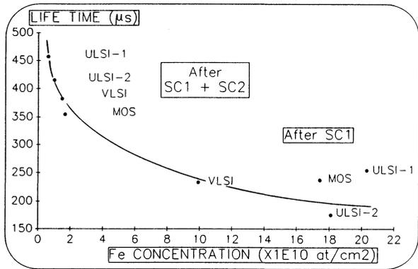
Figure 2 : Correlation between minority carriers MOS lifetime and Iron surface contamination after different RCA cleaning processes : MOS, VLSI and ULSI.
