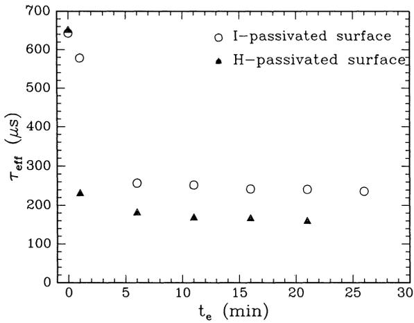
Fig. 5: Superior passivation stability of I vs. H. The wafer is float-zone p-Si(100).  $t_e$  is the time that the wafer was exposed to air.
