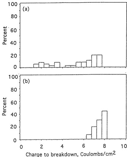
Figure 6, Charge to breakdown characteristics of 105A gate oxide intentionally contaminated with Al prior to the oxidation (a) without and (b) with Pyrochemical cleaning.
