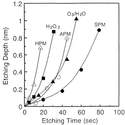
Figure 1. Etching rates of various chemical oxides. The etchant is BHF with 0.1nm/min etching rate for thermal oxide at 25°C.
