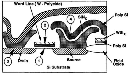
Fig. 1. Applications for HF vapor processing include: 1) Pre-gate Oxidation, 2) Pre-Silicide CVD, 3) Pre-Poly CVD, and 4) Pre-Nitride CVD [1].
