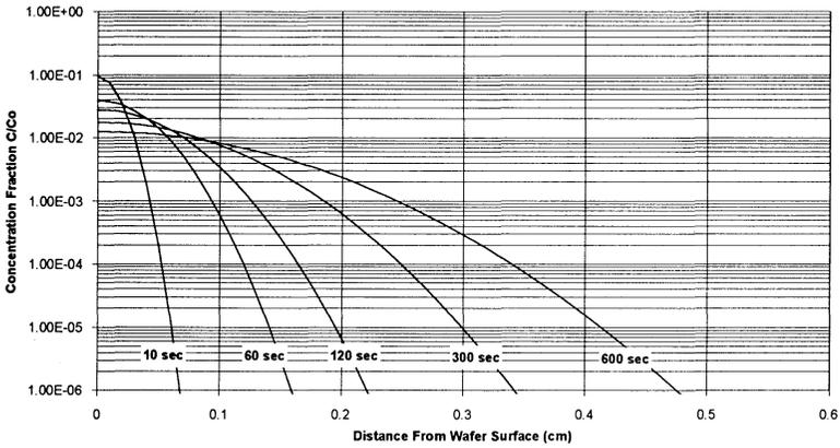
Figure 2. Fractional concentration profile  $C(x,t)/C_0$  for diffusion of residues in a carryover volume of initial concentration  $C_0$  and average thickness of  $20 \mu\text{m}$ .
