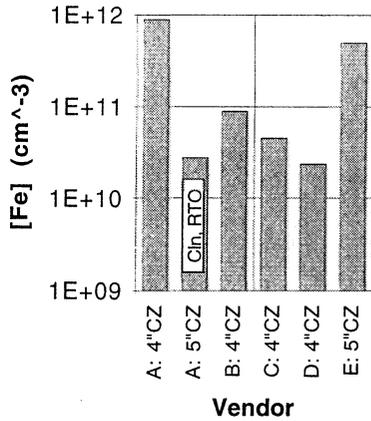
Fig. 4. [Fe] (cm<sup>-3</sup>) obtained on wafers from different sources.
