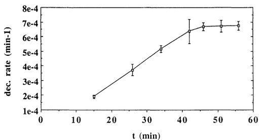
Figure 1: Decomposition rate of a SC1 mixture versus age of the solution (0.25/1/5 at 70 °C, metal levels: < 0.5ppb in total SC1).
