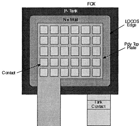
Figure 3: Moat block diode array for junction leakage data collection.
