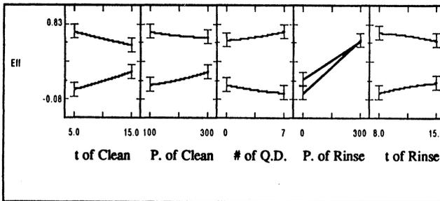
Fig.2. A model graph illustrates the factor-response relationship when each factor interacts with other factors. The top line for each factor shows the most positive effects that factor can have on the response. The bottom line shows the most negative effects that factor can have on the response.
