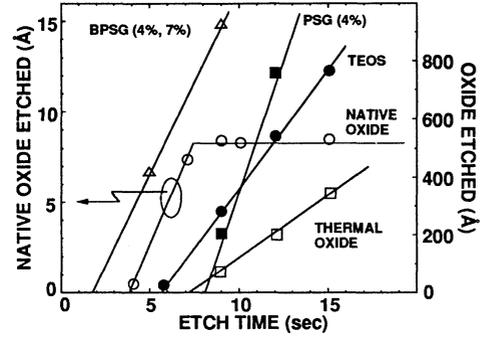
Fig. 2. Etch rate and delay times using azeotropic HF/H<sub>2</sub>O are strongly dependent on the oxide type.
