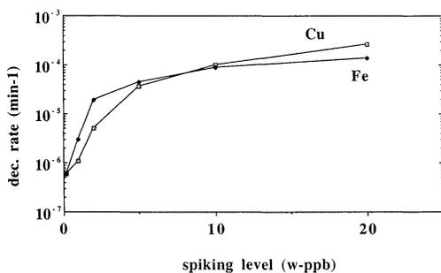
Figure 2: Dependence of the decomposition rate of an ultra pure H<sub>2</sub>O<sub>2</sub> on the Fe and Cu contamination level at 70 °C (all other metals: < 0.4ppb).
