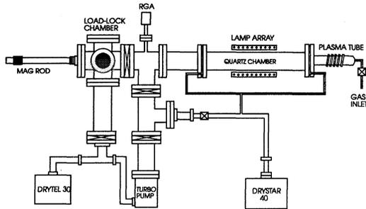
**Figure 1:** Schematic of the dual RTP-RPECVD reactor
