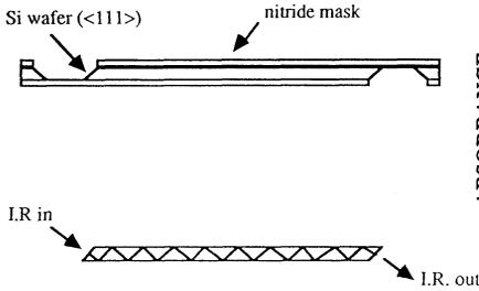
Fig. 1 : Preparation of the MIR silicon crystals by KOH etching of a double side patterned nitride masked wafer (a) and IR light path through the chamfered crystal (b).
