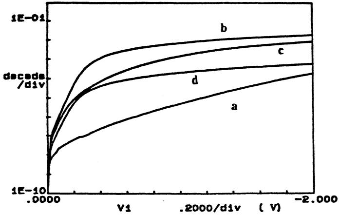
Figure 5. I-V curves for (a) an etched sample, (b) a control sample, (c) an etched and oxygen cleaned sample, and (d) an etched and UV-ozone cleaned sample for the OE  $\text{CHF}_3/\text{CF}_4/\text{Ar}$  case.
