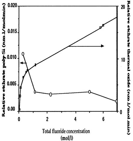
Figure 13 : Relative etch rates for thermal oxide and for poly-Si as a function of the total fluoride concentration for the HF/HCL mixture.
