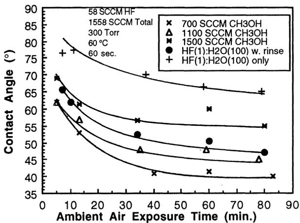
Fig. 4. Contact angle vs. time for different CH<sub>3</sub>OH flow rates.
