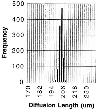
Fig. 1. L measurements of p-type wafer.  $L=204\mu\text{m}$ ,  $N=1100$ ,  $\sigma=2.35\mu\text{m}$ .
