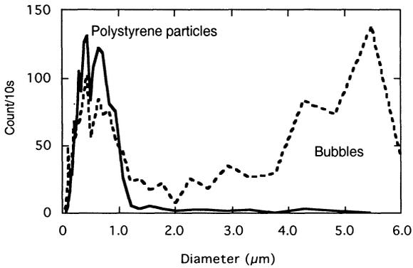
Fig. 5 Distribution of polystyrene particles and bubbles generated by ultrasonication.
