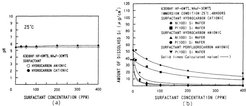
Fig.3 Relationship between the concentration of surfactants and (a) pH and (b) the amount of dissolved Si in 630BHF.
