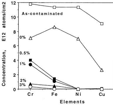
Figure 3. HCl concentration dependency of Pyrochemical cleaning for removal of Fe, Ni, Cr and Cu.
