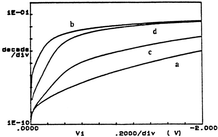
Figure 2. I-V curves for (a) an etched sample, (b) a control sample, (c) an etched and oxygen cleaned sample, (d) an etched, oxygen cleaned and HF etched sample for the RIE  $\text{CHF}_3$  case.
