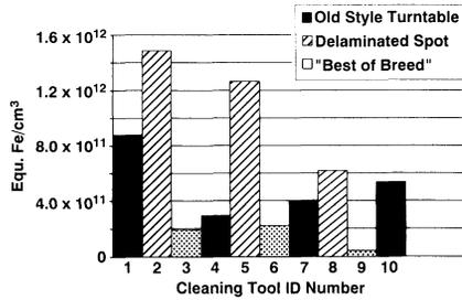
**Figure 4.** Baseline measurements of cleaning tools link average equivalent from concentrations with real tool differences.
