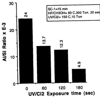
Fig. 6 SIMS results showing changes in Al content as a function of UV/Cl<sub>2</sub> exposure time with preceding oxide etching step.
