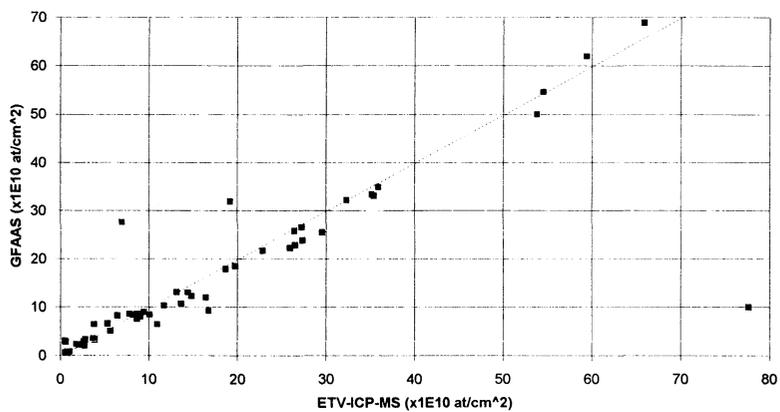
Figure 1. Correlation for Fe Between ETV-ICP-MS and GFAAS on Silicon Wafers.
