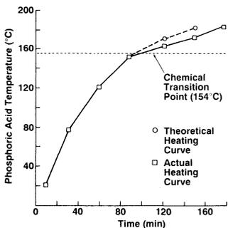
**Figure 1. Phosphoric acid heating characteristics.**
