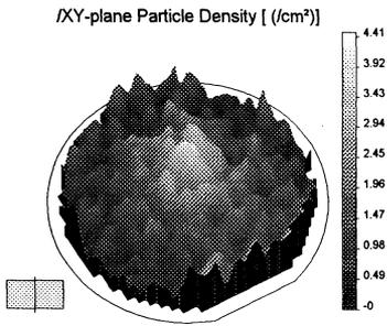
**Figure 5.** The distribution of particles, averaged over one cassette of wafers, after cleaning in a spray post system.
