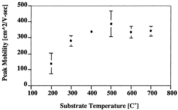
Figure 5. Plot of peak mobility vs. substrate temperature during H-plasma cleaning .
