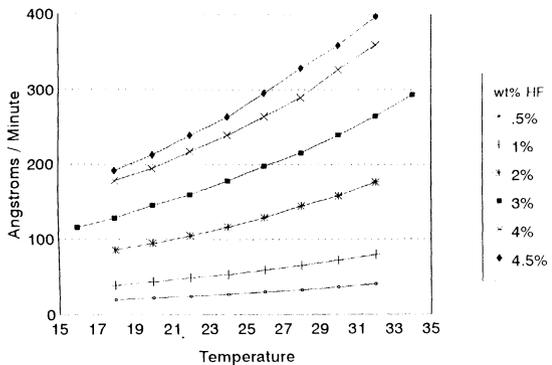
Figure 1. Etch rates of thermal oxide as a function of both HF concentration and bath temperature.
