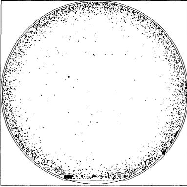
**Figure 8.** Oxidation induced stacking fault distribution (experimental crystal), made visible by a 4 min Wright etch and subsequent LPD scan.
