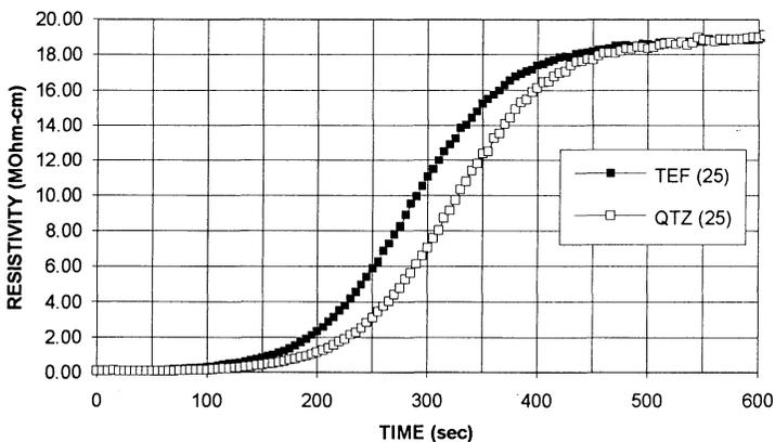
Figure 8. Experimental (points) and calculated (lines) rinse resistivity curves for the Teflon and quartz full cassette in the AWS with 25 wafers.
