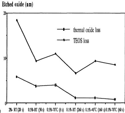
Figure 11 : Thermal oxide and TEOS oxide loss as a function of the process to remove the native oxide (concentration and temperature are varied).
