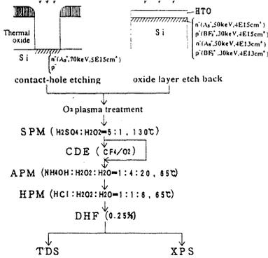
Figure 1 A schematic diagram of Si-surface treatment processes for contact-holes and non-patterned Si surfaces.
