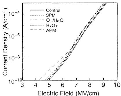
Figure 4. Current density-average oxide field characteristics of MOS diodes with 5nm thick gate oxide films incorporating the chemical oxides formed by various chemicals.
