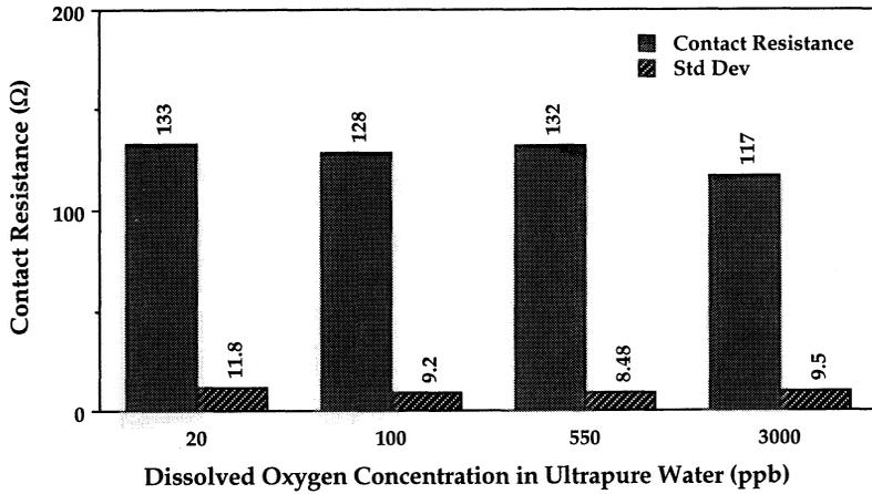
**Figure 5. Contact Resistance as a Function of Dissolved Oxygen**
