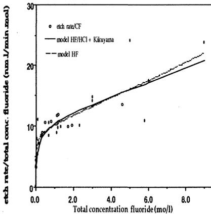
Figure 5 : Measured relative etch rate (dots) and fitted etch rates when the dimerisation reaction is taken into account.
