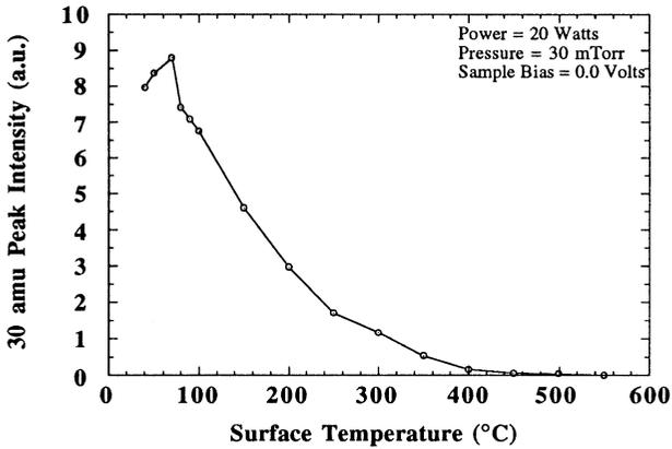
Fig. 1 Temperature dependence of the 30 amu signal from residual gas analysis spectra collected during H-plasma processing.
