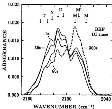
Fig. 8 :  $\text{SiH}_x$  spectrum as a function of etch time in a buffered  $\text{HF}$  solution showing the change of a dihydride to a monohydride covered surface.
