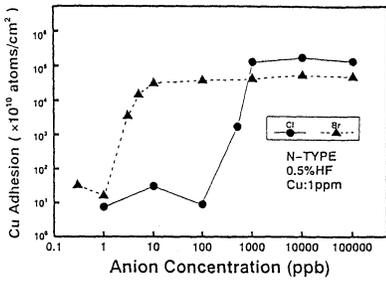
Figure 8 The relationship between the halogen concentration and the Cu adhesion onto n-type Si surface
