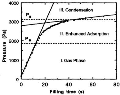
Figure 3. Pressure versus filling time for the isolated reactor. The flow of the 10 % mol HF-H<sub>2</sub>O vapour mixture is constant. The different pressure regimes are indicated by dotted lines.
