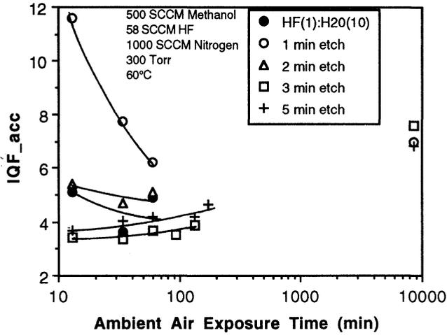
Fig. 5.  $IQF_{acc}$  vs. time for different etch times.
