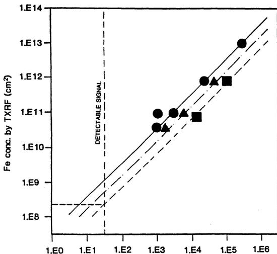
**Figure 3.** Fe counts obtained during TOF-SIMS analysis of silicon wafers using analysis areas of  $65\ \mu\text{m} \times 65\ \mu\text{m}$  (●),  $100\ \mu\text{m} \times 100\ \mu\text{m}$  (▲), and  $150\ \mu\text{m} \times 150\ \mu\text{m}$  (■) versus Fe concentration determined by TXRF. The detection limits are indicated by linear extrapolation through the data points.
