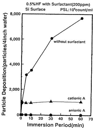
Figure 1 The effect of the addition of surfactant
