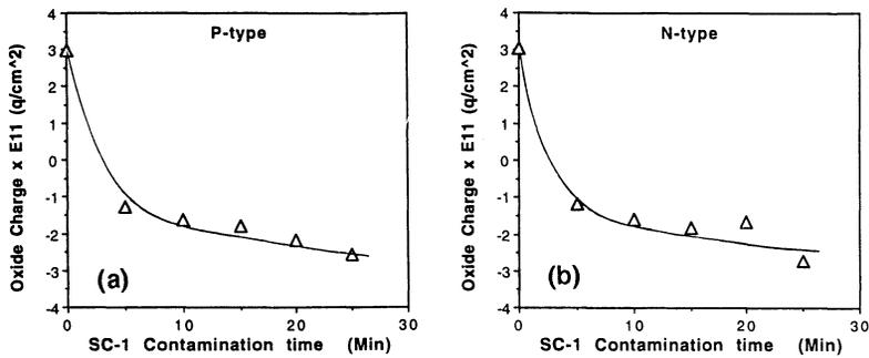
Fig.2 Oxide charge vs. SC-1 immersion time for (a) p-type and (b) n-type Si wafers.
