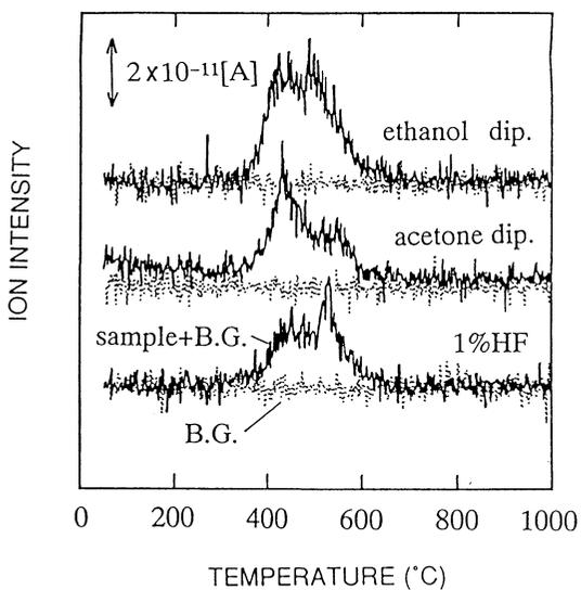
Fig. 8 APIMS-TDS spectra of  $CO_2^-$  measured under flowing oxygen.
