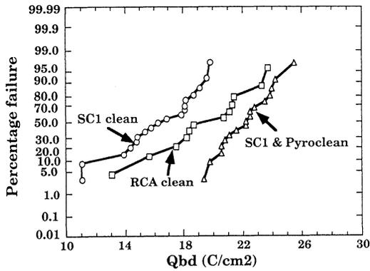
Figure 10, Charge to breakdown characteristics of 105A gate oxide with various pregate cleans.
