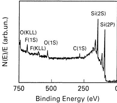
Fig. 4: XPS survey spectrum obtained after etching.
