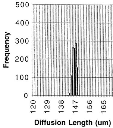
Fig. 2. L measurements of n-type wafer.  $L=146\mu\text{m}$ ,  $N=1100$ ,  $\sigma=1.23\mu\text{m}$ .
