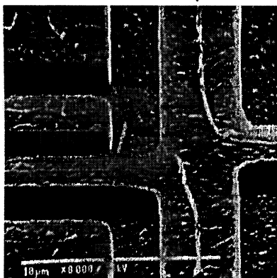
Fig. 3. Veil polymer defects from the plasma metal etch process.
