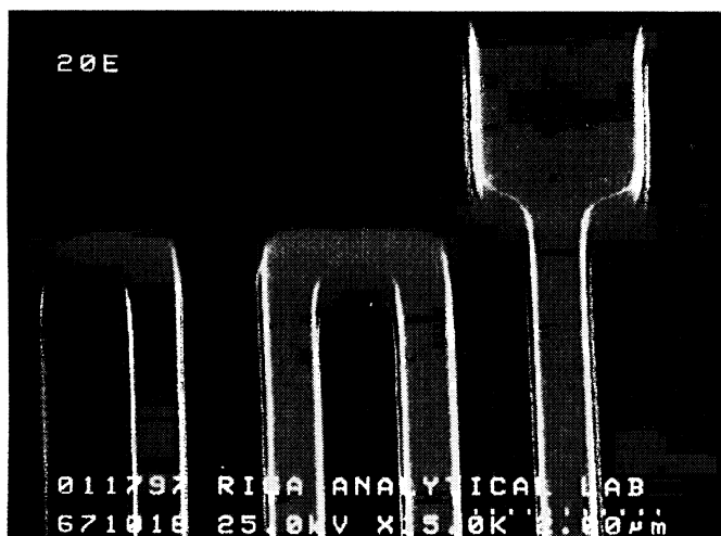
Figure 4. SEM photograph of wafer processed using Test Condition 4: \text{O}_3 injected into the DI rinse water and no intermediate rinse.
